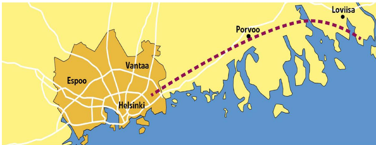
Figure II.5.1: Heat transportation system routing from the Loviisa 3 NDH unit to the Helsinki metropolitan area, about 80 km long. Data sources: ISNP, 2014.
