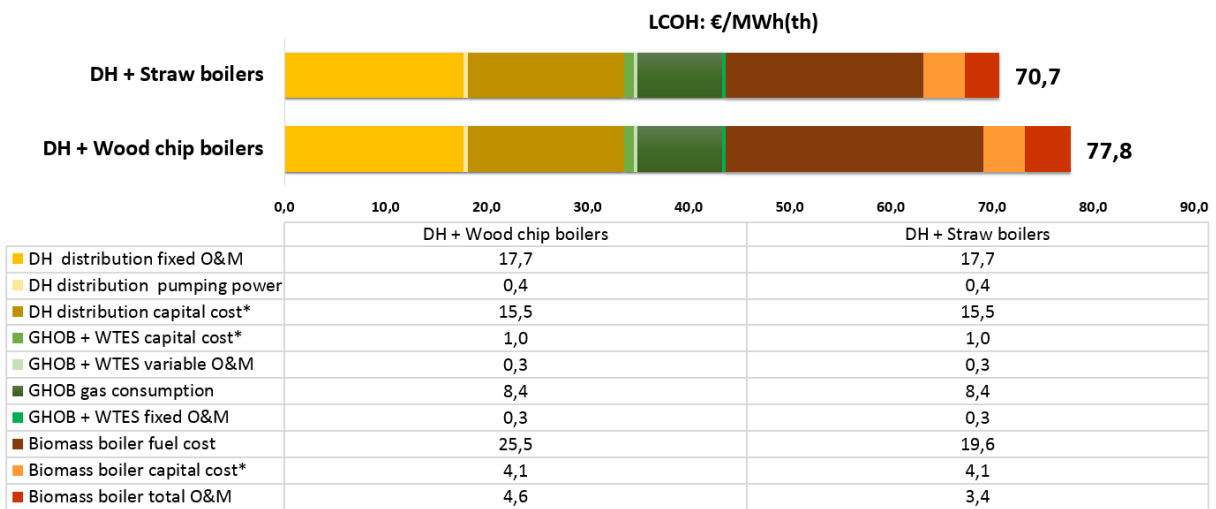
Figure I.3.16: LCOH breakdown of the DH + Biomass HOB systems (see Section 4.1.1.5 for assumptions).
