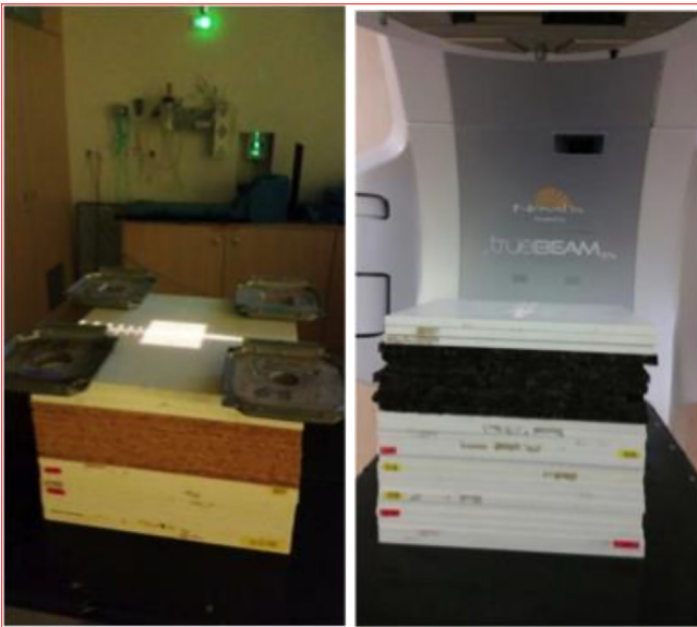
Fig. 2. Heterogeneous (PMMA/cork) phantoms to study dose distributions in DIBH (right) and FB (left) patients. Cork densities are 0.24 (left) and 0.12 g.cm -3 (right).
