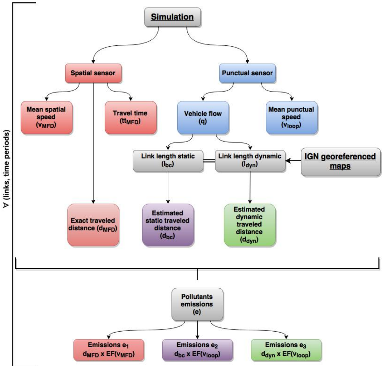
Fig. 2.5 – The traffic variables recovered from each link and time period of the network and their respective emission calculations.
