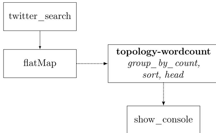
Figure 5.7 – Representation of the Twitter Wordcount with a topology-wordcount sub-graph.
