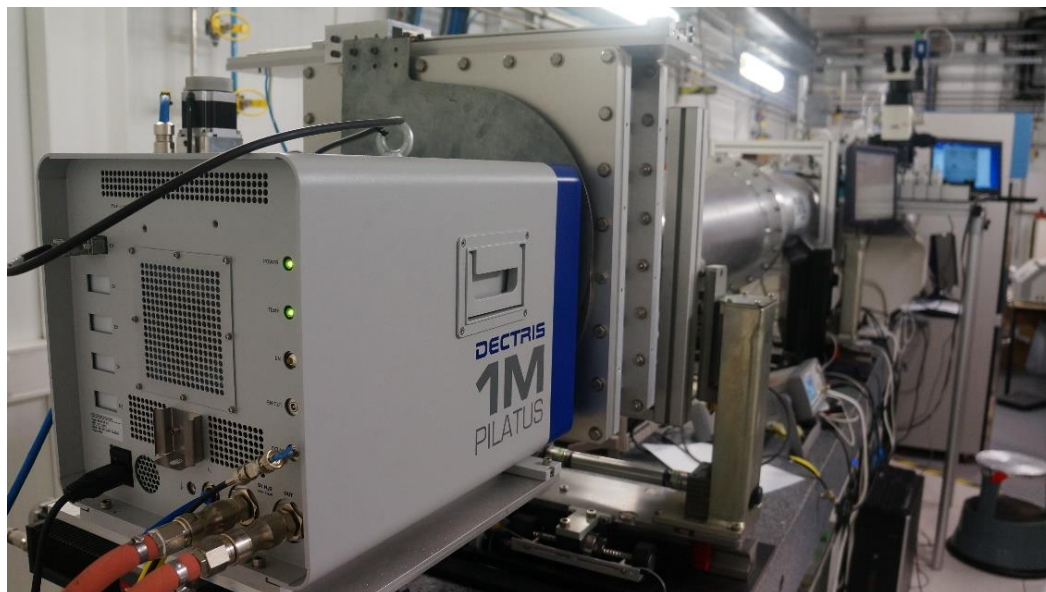
Figure III-13: Pilatus 1M at the moment is the best detector for solution SAXS- Beamline 29 ESRF Grenoble - France
