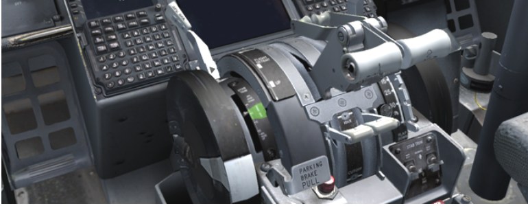
Figure 32: Throttle console of a Boeing 737 used in takeoff rejection procedure
