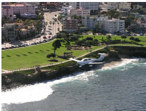
Figure C – Diamond Star DA40 aircraft (three-blade propeller, 180 shaft horse power). Taken from scripps.ucsd.edu/labs/buckingham/research/aircraft-sound .
