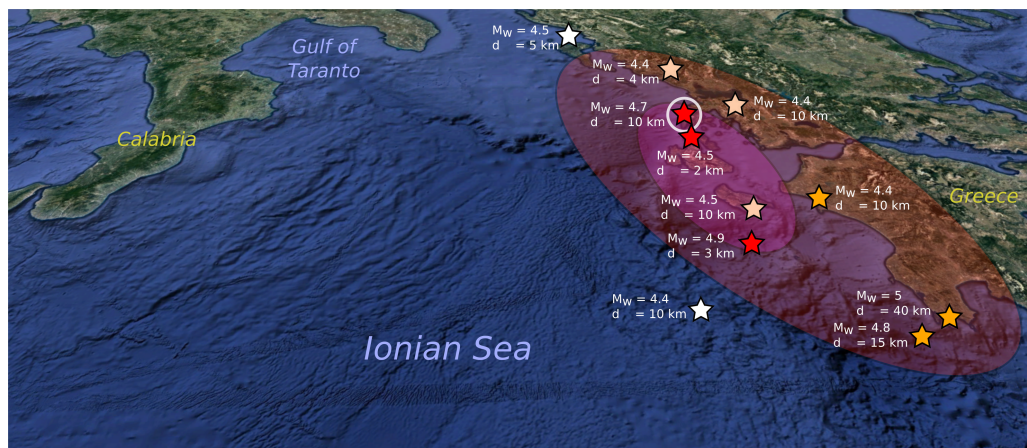
Figure 2.5 – For each earthquake indicated on the above map (star), both the characteristics from NOAA (magnitude and hypocenter depth d ) and the quality of the generated T-waves are detailed. The classification has been made from the same kind of map than the one presented in Figure 2.1. Red stars: more than 5 Italian stations have recorded strong T-phases ("red" stations), orange stars: some Italian stations have recorded strong T-phases, light orange stars: T-phases recorded by several Italian stations, white stars: no T-waves visible. Earthquakes occurring in the red area are prone to generate T-waves. Earthquakes occurring in the purple area are particularly prone to generate strong T-waves. That area corresponds to the Greek peninsula of Paliki. The circle indicates the earthquake shown above.
