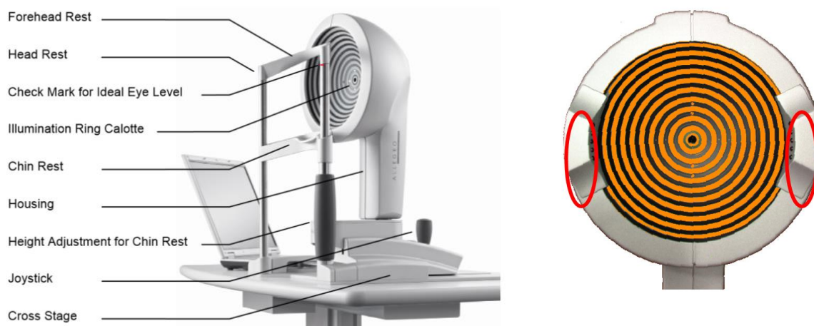
Figure 2: Optics Unit Design
