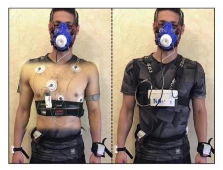
Figure 3.4 - A participant wearing the sensors and gas exchange system. Some sensors must be placed in direct contact with the skin as seen in the picture on the left while others are worn on top of the clothes as seen in the picture on the right.
