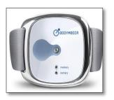
The BodyMedia armband is a multi-sensor device designed to be worn at the left upper arm over the triceps. The integrated sensors deliver triaxial acceleration measures and a variety of physiological variables: the heat flux, the skin temperature, the near-body ambient temperature, the galvanic skin response. This multi-sensor armband was conceived as an EE assessment tool. The manufacturer's software permits to study the type and the intensity
