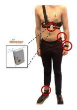
Figure 3.1 - The Shimmer sensor nodes and the ECG electrodes positions on the body in the basic protocol.
