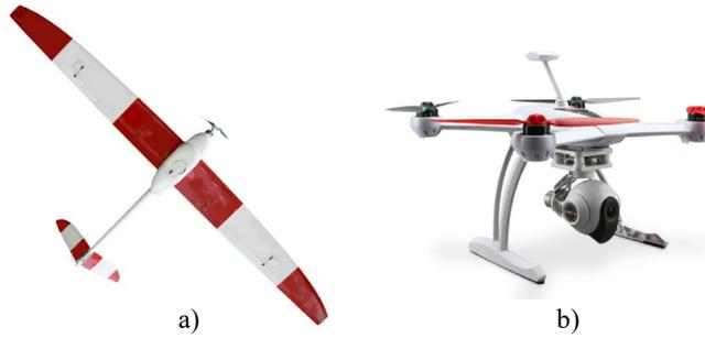
Figure 2-5. Two categories of UAVs: a) Fixed-wing b) Rotary-wing
