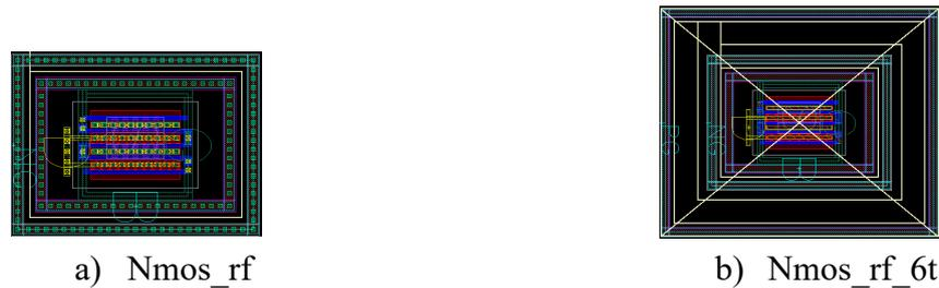
Figure 4-12. Layout of two transistor models `nmos_rf` and `nmos_rf_6t` with deep N well layer
