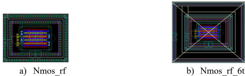
Figure 4-12. Layout of two transistor models nmos_rf and nmos_rf_6t with deep N well layer
