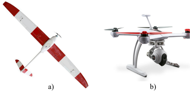
Figure 2-5. Two categories of UAVs: a) Fixed-wing b) Rotary-wing
