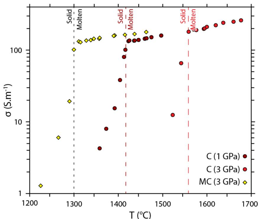
**Figure 3. Electrical conductivity vs. temperature showing the melting temperature of  $\text{CaCO}_3$  and  $\text{MgCa}(\text{CO}_3)_2$  deduced in this study.** Dashed lines indicate melting temperatures determined in previous phase diagram studies from Wyllie and Lee (1998) for dolomite at 2.7 GPa and Suito et al. (2001) for calcite at 1 and 3 GPa.
