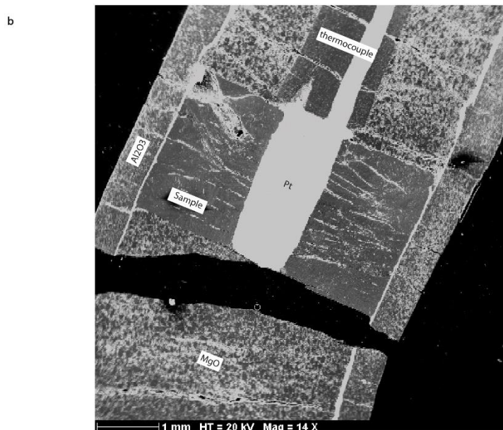
Extended Data Figure 1. a, Modified piston cylinder assembly for electrical conductivity measurements using a 4-wires configuration. The cored sample (in green) contains in its centre an inner electrode in platinum (in blue). A platinum foil (in blue) surrounds the sample, which extends upwards and downwards from the sample and corresponds to the outer electrode. The sample is sandwiched by machined MgO ceramics (in white). The electrode-sample assemblage is isolated from the graphite furnace by an Al 2 O 3 jacket (in yellow). The 4-electrode wires are emplaced using a 4-hole Al 2 O 3 tube (in orange). Two of these wires, i.e. the thermocouple, are in contact with the inner electrode, whereas the outer electrode is in contact with two other wires by means of a top Ni plug (in red). b, SEM image of the assemblage of sample C after experiments (up to 1463°C and 3 GPa). We observed an average decrease of 20% compared to the initial cell geometry (corresponding to the porosity loss during melting). Cell geometry parameters ( h and r_{in} , r_{out} in equation SI2) are determined from SEM images for each sample.
