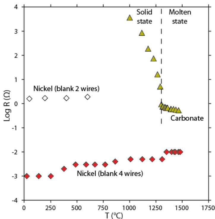
**Figure 2. The electrical cell resistance versus temperature at 3 GPa.** We show the resistance of a sample made of nickel measured using either a 2-wire setup (empty diamond) or a 4-wire setup (red diamond). There are several orders of magnitude difference between the two measurements showing that the 2-wire setup is not suitable for conductive materials. The resistance of sample MC is also shown in 4 wires setup.
