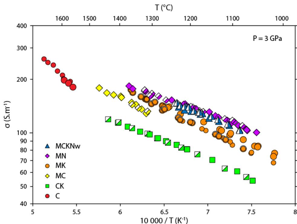
**Figure 4. Measured electrical conductivity vs. temperature of molten carbonates during heating (full symbols) and cooling cycles (half empty symbols). Error on the plotted electrical conductivities is within  $\pm 10\%$ . Sample C present two**
