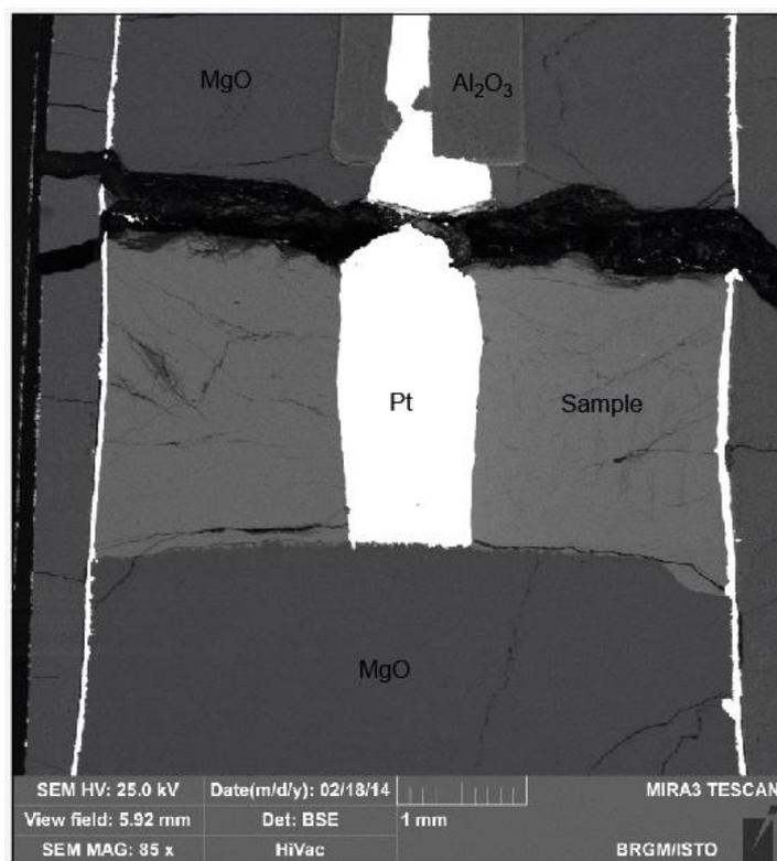
**Figure S1.** SEM image of sample C after experiment (up to 1497°C and 1 GPa). Porosity loss during melting was observed leading to an average decrease of 20% compared to the initial cell geometry. The cell geometry parameters ( $r_{in}$ ,  $r_{out}$  and  $h$  from equation 1) are determined from SEM images for each experiment.
