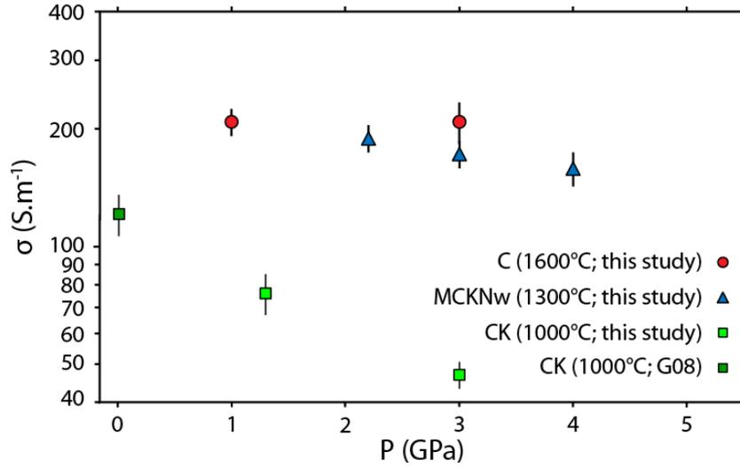
**Figure 5.** Measured electrical conductivities as a function of pressure for samples C at 1600°C, MCKNw at 1300°C and CK at 1000°C. Run CK at 1000°C and 0 GPa is from the study of Gaillard et al. (2008).
