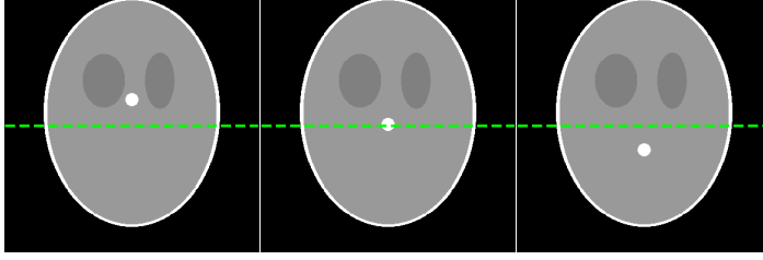
Figure 24: Simulation of a non-rigid motion. A sphere of radius 4 mm is displaced, starting in projection 47, traversing the central line, and ending at projection 65.
