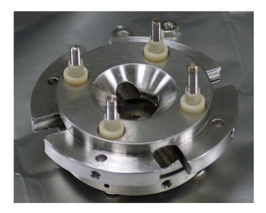
Fig. 1.2: Photo of the hyperbolic Paul trap from our team. Stainless steel hyperbolic trap made of a ring electrode with an hyperbolic shape and two endcaps (the top one is missing). The white ceramics ensure electric insulation between the different electrodes. Note the holes in the ring electrode used for molecular beam intake and UV irradiation.
