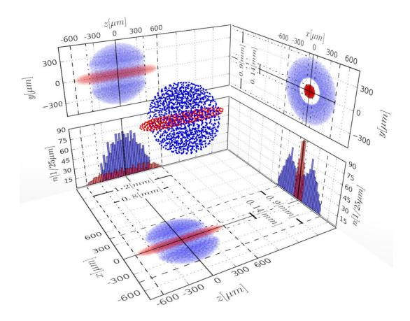
Fig. 4.4: Coulomb crystal composed of 1469 Be<sup>+</sup> and 450 H<sub>2</sub><sup>+</sup> with  $a_x = 5.25 \times 10^{-7}$ ,  $q_x = 0.0223$  for the Be<sup>+</sup> and  $\hat{\omega}_z = 250$  kHz. Characteristic lengths are given along with linear density n. By courtesy of J. Heinrich [31].
