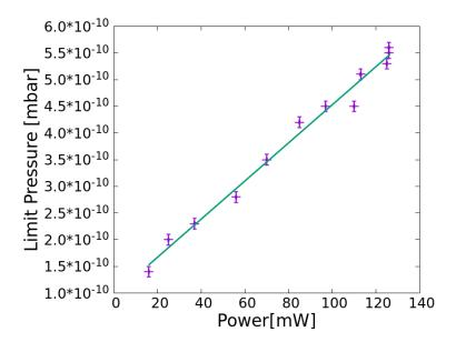
Fig. 3.6: Limit pressure in the trap chamber after continuous exposition to different powers of the 213 nm laser dissociation laser. The solid line is a fit of the form  $\eta P_{total} + c_1$  with  $\eta = 3.6 \times 10^{-12} \pm 1 \times 10^{-13} \, \mathrm{torr} \, \mathrm{mW}^{-1}$  and  $c_1 = 1 \times 10^{-10} \pm 1 \times 10^{-11} \, \mathrm{torr}$ .
