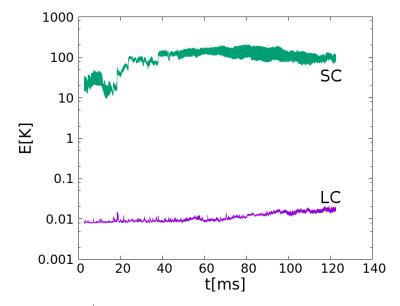
Fig. 5.3: Energy of an  $\bar{\rm H}^+$  starting at 3.125 meV sympathetically cooled by a crystal of 1919 Be<sup>+</sup>. After 120 ms the  $\bar{\rm H}^+$  has actually heated up to about 8.6 meV while the Be<sup>+</sup> has also heated up by a factor of about 2. Other parameters as in Fig. 4.5.
