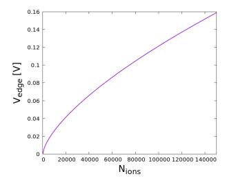
Fig. 1.7: Value of the potential, for an ion of charge 1 e, at the edge of a spherical crystal composed of ions of charge 1 e as a function of the number of ions, with  $\hat{\omega}_z = 2\pi \cdot 250 \,\text{kHz}$  using Eq. 1.36.
