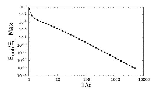
Fig. 4.8: Ratio of the energy of a projectile ion after and before a 1D collision with a stationary target ion of equal mass as a function of the  $\alpha$  parameter in the variable timestep criterion described in Eq. 4.26. As  $\alpha$  decreases the simulation approaches the analytical result (for infinite initial distance) of complete energy transfer between the projectile and the target ions of equal mass.
