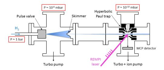
Fig. 2.4: Schematic of the  $H_2^+$  ion source design. Pulses of  $H_2$  gas pass through a skimmer to be photo-ionized by the REMPI laser and state-selectively produce  $H_2^+$  in the trap.
