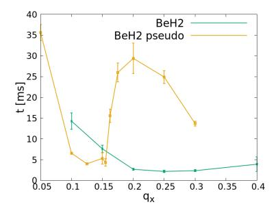
Fig. 5.14: Capture time versus  $q_x$  for an  $\mathrm{H}_2^+$  ion initial energy of 21.25 meV. When the radial stability parameter  $q_x$  is changed, the axial trapping is adapted to keep the shape of the crystal constant. The "BeH2 pseudo" curve corresponds to the data of Tab. 5.5 while the "BeH2" curve corresponds to the data of Tab. 5.3. Error bars are taken to be the standard deviation divided by the square root of the number of simulations.
