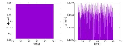
Fig. 4.10: The situation is identical to Fig. 4.9 except that the ion has more radial motion energy and we look at the conservation of that energy by looking at the amplitude of motion along x. Other parameters as in Tab. 4.2.
