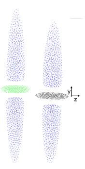
Fig. 5.7: Left: Image of the asymmetric  $\mathrm{Be^+}$ ,  $\mathrm{HD^+}$  crystal which was used in the simulations of Fig. 5.5. Right: Image of the asymmetric  $\mathrm{Be^+}$ ,  $\mathrm{H_2^+}$  crystal which was used in the simulations of Fig. 5.11.  $\mathrm{Be^+}$  is in blue,  $\mathrm{H_2^+}$  in black and  $\mathrm{HD^+}$  in green.
