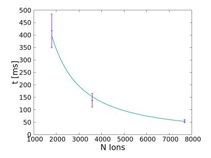
Fig. 5.19: Capture time of a 125 meV  $\bar{\rm H}^+$  in crystals composed of different ion numbers with approximately 20% HD<sup>+</sup> and 80% Be<sup>+</sup>. The full line is a fit of the form  $c_1 N_{Ions}^{c_2}$  with the fitting parameters found to be  $c_1 = 1.3 \times 10^7 \pm 9 \times 10^6$  ms and  $c_2 = -1.38 \pm 0.09$ .  $\hat{\omega_z} = 250 \, {\rm kHz}, \, q_x = 0.2$  for the  $\bar{\rm H}^+$  and other parameters described in Tab. 5.8.
