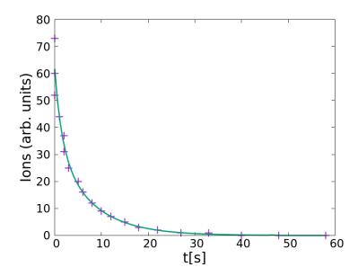
Fig. 3.7: After 2s of creation by electron gun,  $H_2^+$  ions are extracted for detection by the MCP. Ion signal versus extraction time is plotted and fitted (solid line) with Eq. 3.22 with  $A=32\pm22,\ B=0.13\pm0.06\,\mathrm{Hz},\ C=0.6\pm0.7$  and  $\beta=2.5\pm2.9\,\mathrm{s}$ . The 213 nm dissociation laser is off.
