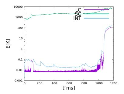
Fig. 5.20: One of the simulations for a  $125\,\mathrm{meV}\ \bar{\mathrm{H}}^+$  in a crystal of  $2883\,\mathrm{Be}^+$  and  $700\,\mathrm{HD}^+$ , in which heating occurs instead of sympathetic cooling. Parameters given in Tab. 5.8. As the heating occurred Be<sup>+</sup> ions started heating up and touching the electrodes (therefore being removed from the simulation), wich aggravated the situation.
