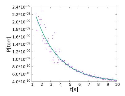
Fig. 3.4: Zoom on the beginning of Fig. 3.3 up to  $10 \,\mathrm{s}$  (right). The solid line is a fit of the form  $c_1 + e^{-\frac{t}{\beta}} + c_2$  with  $\beta = 2.5 \pm 0.1 \,\mathrm{s}$ ,  $c_1 = 3.2 \times 10^{-9} \pm 1 \times 10^{-10} \,\mathrm{torr}$  and  $c_2 = 3.8 \times 10^{-10} \pm 2 \times 10^{-11} \,\mathrm{torr}$ .
