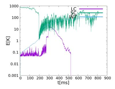
Fig. 5.9: Energy of a 125 meV  $\bar{\rm H}^+$  in green being sympathetically cooled by a crystal of 991 Be<sup>+</sup> in purple and 800 HD<sup>+</sup> in blue. The purple curve going to 0 around 500 ms corresponds to loss of all the Be<sup>+</sup> in the trap. Other parameters as in Fig. 5.5.
