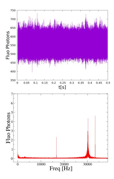
Fig. 5.17: Fluorescence photons(top) and its Fourier transform(bottom) from Be<sup>+</sup> in a crystal of 1441 Be<sup>+</sup> and 350 HD<sup>+</sup> as it cools down a  $\bar{\rm H}^+$  ion with an energy of 125 meV. Fluorescence points are  $1\times 10^{-7}\,{\rm s}$  apart. Trapping parameters are identical to Fig. 5.5.
