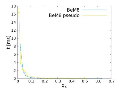
Fig. 5.12: Capture time versus  $q_x$  for a mass 8 ion with an initial energy of 21.25 meV. When the radial stability parameter  $q_x$  is changed, the axial trapping is adapted to keep the shape of the crystal constant. The "BeM8 pseudo" curve corresponds to the data of Tab. 5.6, "BeM8" to Tab. 5.4. Error bars are taken to be the standard deviation divided by the square root of the number of simulations.
