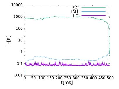
Fig. 5.6: Energy of a 125 meV  $\bar{\rm H}^+$  in green being sympathetically cooled by a crystal of 1441 Be<sup>+</sup> in purple and 350 HD<sup>+</sup> in blue with parameters as in Fig. 5.5. "INT" refers to the auxiliary ions with an intermediate mass in between that of the laser-cooled and the sympathetically-cooled species used to improve mechanical coupling.
