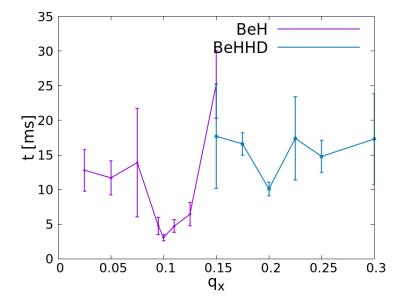
Fig. 5.13: Capture time versus  $q_x$  for an  $\bar{\mathrm{H}}^+$  ion. When the radial stability parameter  $q_x$  is changed, the axial trapping is adapted to keep the shape of the crystal constant. The "BeH" curve corresponds to the data of Tab. 5.2 (3.125 meV) while "BeHHD" curve corresponds to the data of Tab. 5.7 (31.25 meV). Error bars are taken to be the standard deviation divided by the square root of the number of simulations.
