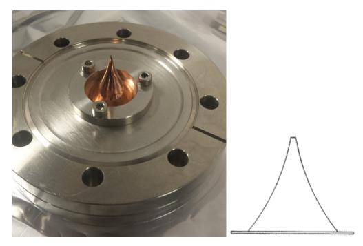
Fig. 2.2: Left: Copper skimmer with an opening of 150 μm mounted onto a CF-63 to CF-40 adaptor flange. Right: Schematic representation of the skimmer.
