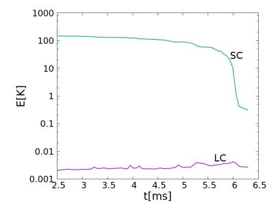
Fig. 5.4: Energy of a 21 meV  $\bar{\rm H}^+$  in green as it gets captured by a crystal of 1919 Be<sup>+</sup> in purple under the pseudopotential approximation.  $a_x=0.00047,$   $q_x=0.31$  for the  $\bar{\rm H}^+,\,\hat{\omega_z}$  and other parameters as in Fig. 5.2.
