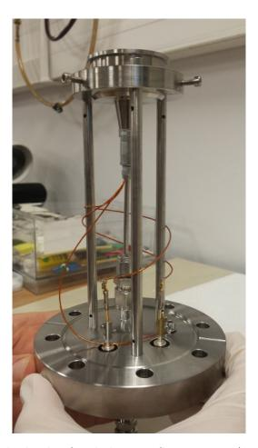
Fig. 2.3: ACPV2 pulsed valve (made by MassSpecpecD BV) mounted onto a CF-63 flange with gas and BNC feedthroughs. The diameter of the valve is  $150\,\mu\text{m}$ , pulse duration is between  $5\,\mu\text{s}$  and  $200\,\mu\text{s}$  and the valve can be operated at up to  $5\,\text{kHz}$ .
