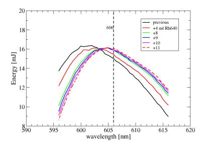
Fig. 2.7: Energy curve of the dye laser, before frequency doubling, as we added millilitres of Rhodamine-640 solution to the previously used dye mixture. The solution of the "+11" curve  $(0.088\,\mathrm{g\,L^{-1}}$  of Rhodamine-610 and  $0.032\,\mathrm{g\,L^{-1}}$  of Rhodamine-640) is what we used in our experiments until we broke a dye cell. Afterwards we used a more dilute solution (concentrations given in text).
