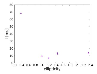
Fig. 5.1: Capture time t of a 62.5 meV mass 8 ion as a function of the ellipticity  $\frac{\omega_x}{\omega_z}$  of a spheroid Be<sup>+</sup> crystal. An ellipticity of 1 corresponds to a sphere, superior to 1 corresponds to a prolate crystal and inferior to 1 corresponds to an oblate (pancake-shaped) crystal.  $\Omega = 13 \,\mathrm{MHz}, \, r_0 = 3.5 \,\mathrm{mm}$ . Data and other parameters in Tab. 5.1.
