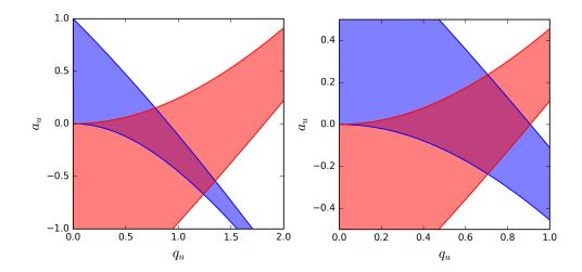
Fig. 1.4: Left: Stability diagram of a hyperbolic Paul trap. The red and blue areas respectively represent the stability regions for the motion along the axial (z) and radial (x, y) directions. 3D trapping is therefore achieved in the intersection of these two areas. Right: Stability diagram of a linear Paul trap. Here the red and blue areas correspond to the x and y directions respectively. By courtesy of J. Heinrich [31].
