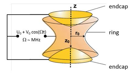
Fig. 1.3: Representation of the electrodes of a hyperbolic Paul trap. The ring electrode is at potential  $V = U_0 + V_0 \cos{(\Omega t)}$  while the endcap electrodes are grounded. The curvature of the electrodes is hyperbolic.
