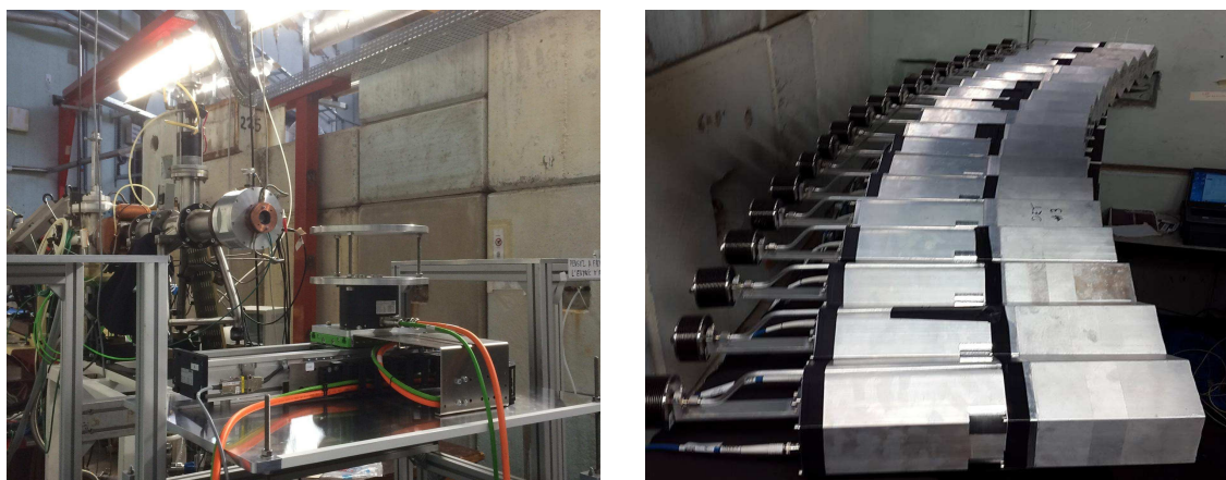
Figure 2.15 – Experimental setup of fast neutron tomography by using LICORNE neutron source, including a scanning table (left) and a neutron detection array NEDA (right).
