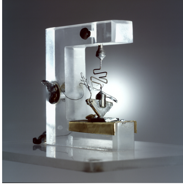
Figure 4.1: First transistor built in 1947 by Shockley, Bardeen and Brattain (picture taken from the web [104]).
