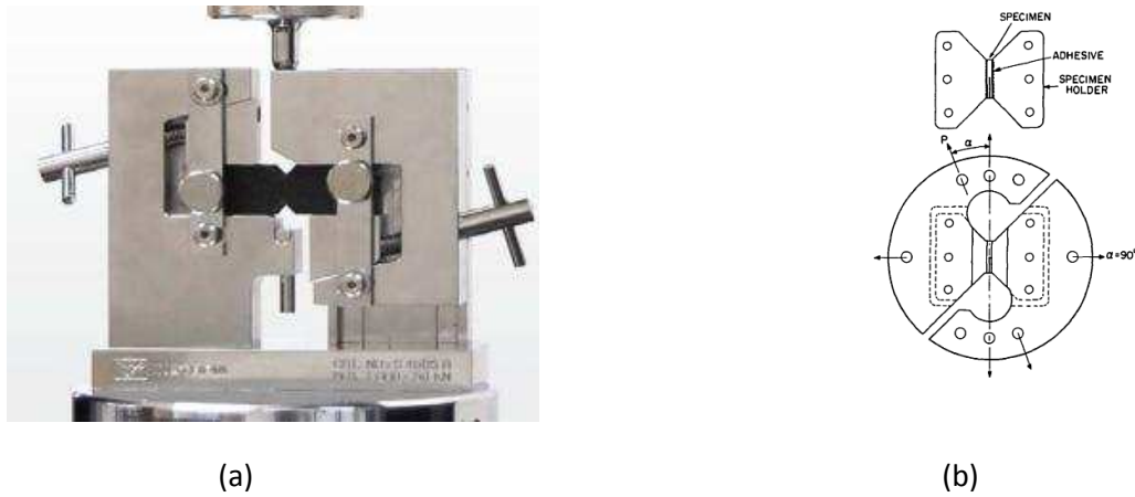
Figure 44. (a) Iosipescu shear test [INSTRON] and (b) Arcan specimen [ARC 87] (reproduced from [ARN 14a]).
