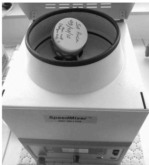
Figure 59. Mixing of epoxy resin and hardener process [SPE].
