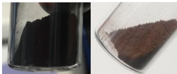
Figure II-16. Left: SMS-derived amorphous boron, kept under argon atmosphere. Right: commercial amorphous boron from ABCR. Containers have a 1 cm diameter.
