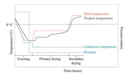
Fig. 2. Freeze-drying cycle, showing shelf, product and condenser temperatures, and chamber pressure. Figure adapted from (Franks, 1998).
