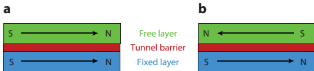
Figure 1.4: The Magnetoresistance Junction device has a ) low- and b ) high- resistance corresponding to the orientations of magnetization in two ferromagnetic layers: parallel and anti-parallel, respectively.
