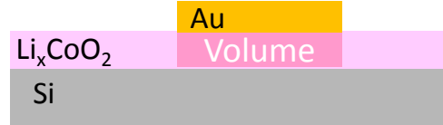
Figure 4.6: The film modification is only considered in the {(top electrode surface) x (film thickness)} volume
