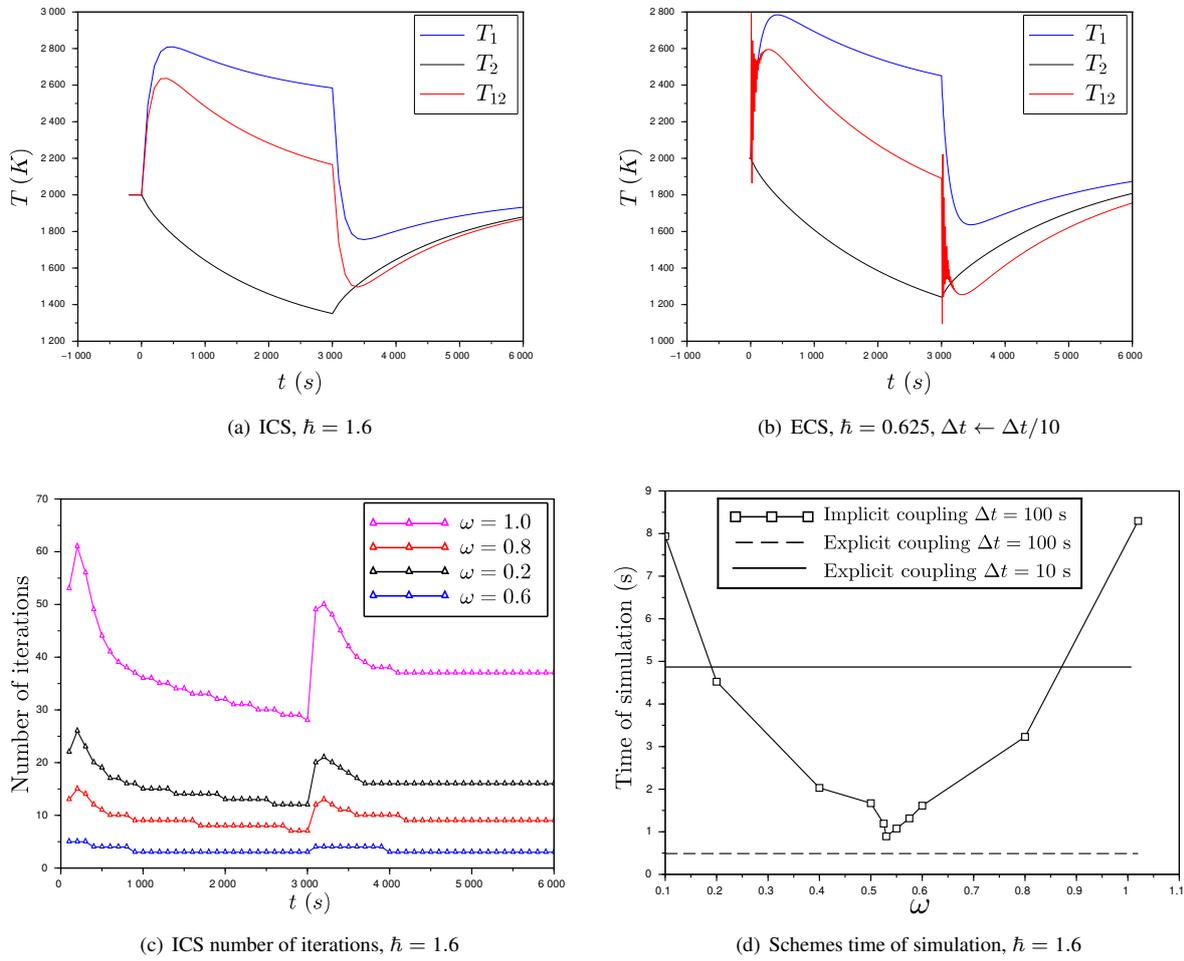
**FIG. 7:** Propagation of discontinuities at boundaries of lumped parameter heat conduction coupled solvers solved with an ICS (upper left) and an ECS (upper right) with much smaller coupling time step.
