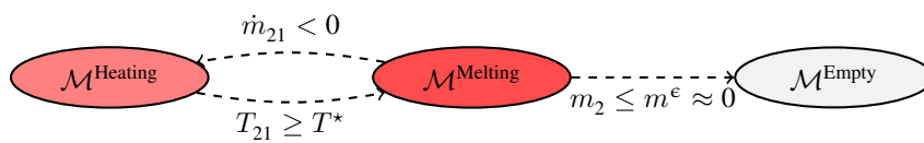
FIG. 8: Internal states of domain \Omega_2 and their transition functions.
