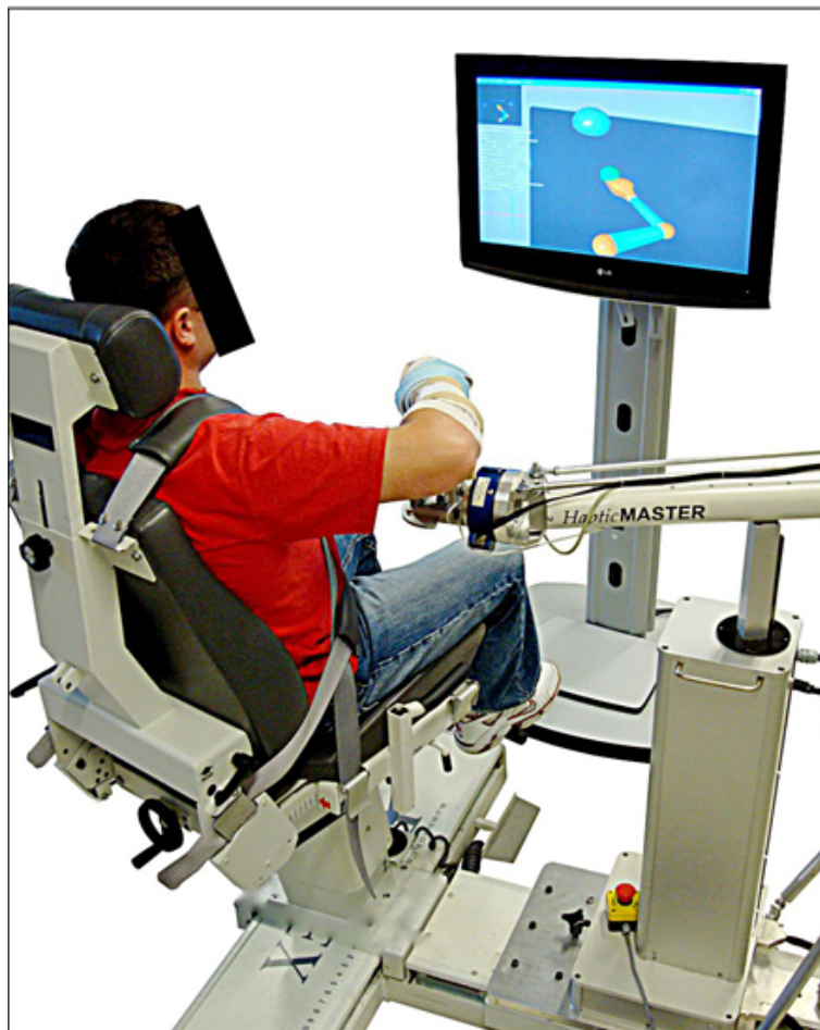
Figure 1.22: Arm Coordination Training 3-D (ACT 3D) robotic system [99]
