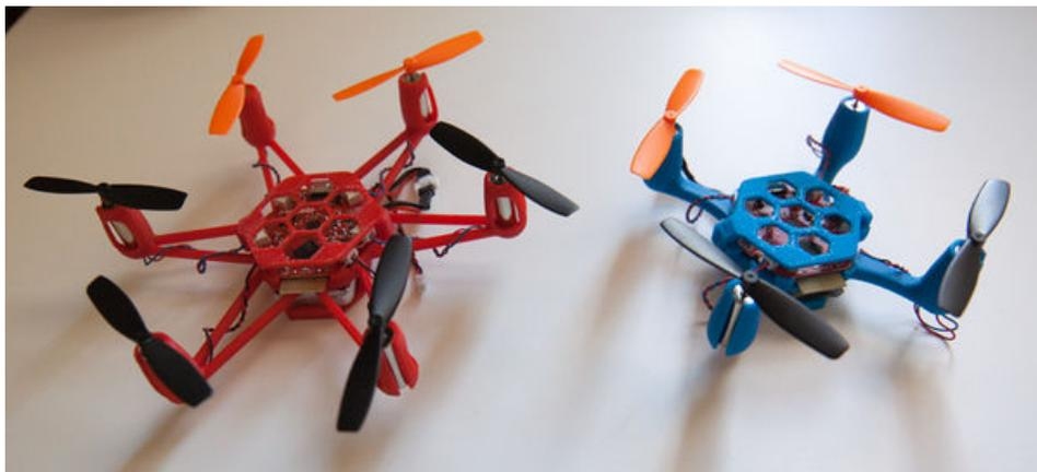
Figure 5.6: Flexbot platform, hexarotor and quadrotor.
