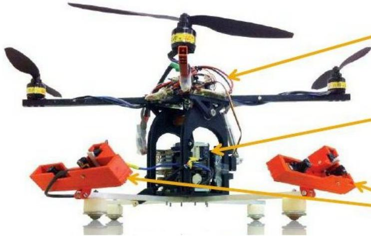
Figure 1.2: Picture of the platform Hybrid quadrotor structure developed by Thorel *et al.*
