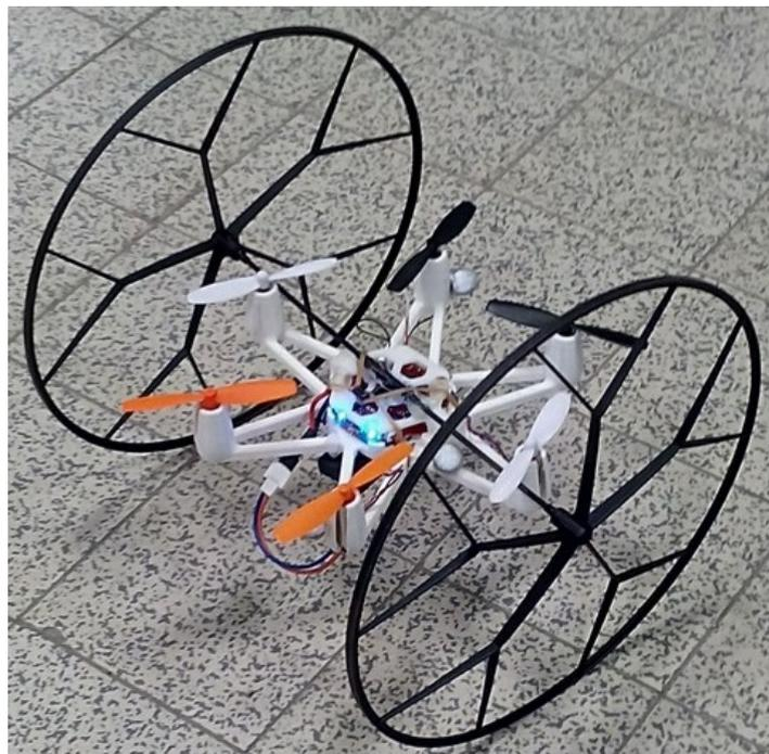
Figure 5.8: Hybrid vehicle using a Hexa-Flexbot.
