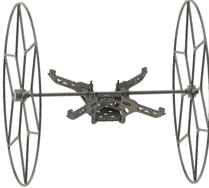
Figure 1.5: Design of the hybrid vehicle prototype.
