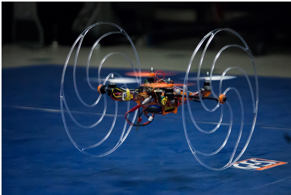
Figure 5.9: Hybrid vehicle using a Multiwii Crius Card.
