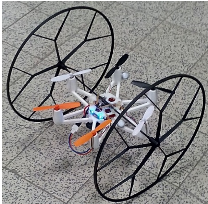
Figure 5.8: Hybrid vehicle using a Hexa-Flexbot.
