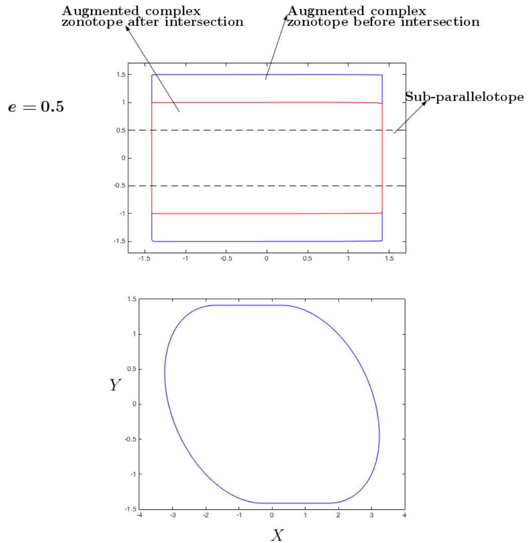
Figure 3.2: Over-approximation of intersection for  $e = 0.5$ .
