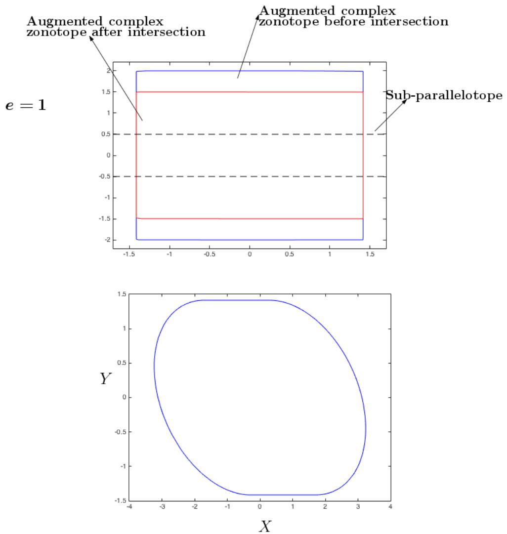
Figure 3.3: Over-approximation of intersection for  $e = 1$ .
