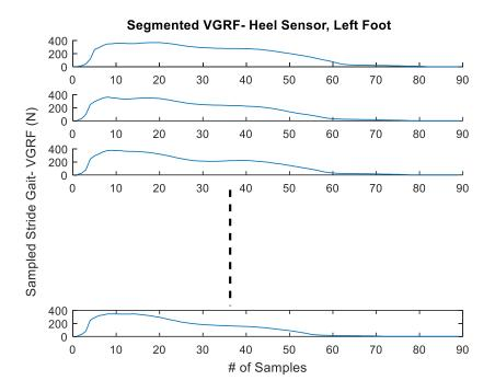
Figure 4.10: Step Isolation of VGRF stance phases at the heel. They are saved over 89 samples equivalent to 0.89 seconds.
