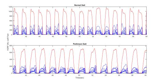
Figure 2.2: Sample of VGRF data captured by the eight sensors underneath the left foot. The red curve represents the resulting signal of their summation. The first row corresponds to normal gait and second raw corresponds to Parkinson gait subject
