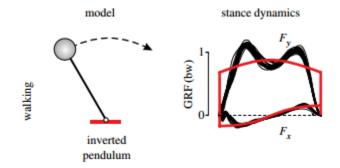
Figure 1.2 Standard conceptual models of legged locomotion. The inverted pendulum is a standard model for walking. The model-predicted stance dynamics (red lines) fit experimental data (black traces recorded from human treadmill walking). Horizontal and vertical ground reaction force (GRF) normalized to body weight (bw).
