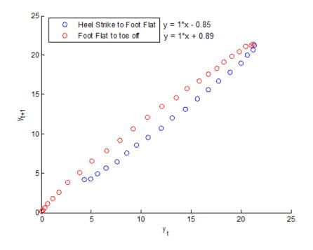
Figure 4.8: Linearity in the plot of current values versus past values in VGRF's data for midsensor on a single step. In this case the difference is one time lag. Given ( $y = y_t$ ) and  $(x = y_{t-1})$  in equations.
