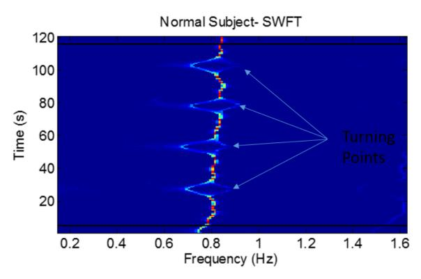
Figure 3.10: synchrosqueezed short time Fourier transform
