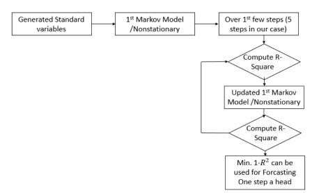
Figure 4.19. Algorithm for Modified Markov Model
