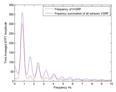
Figure 3.17: The power of frequency content present in tVGRF and the summed amplitude is different from the summation of frequencies for sensor's VGRF.
