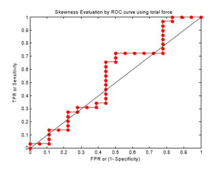
Figure 3.25. Skewness is extracted from the total force from sensors located under the right foot and its performance in binary classification is evaluated using ROC curve
