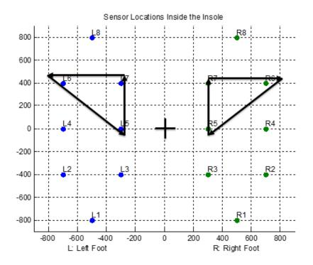
Figure 3.26: The most important locations to acquire data for Gait analysis.
