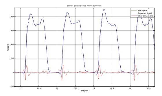
Figure 3.2: Ground Reaction Force filtering by second order Butterworth filter of 25 Hz shows a vital part being attenuated colored in red
