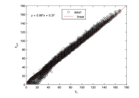
Figure 4.9: Linearity in the plot of current values versus past values in VGRF's data for midsensor given the 2 min signal.
