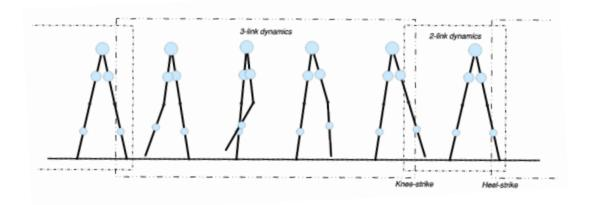
Figure 1.4: Limit cycle trajectory for kneed walker
