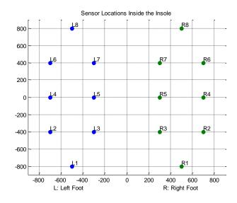
Figure 2.1: Sensor's position as distributed underneath both feet.
