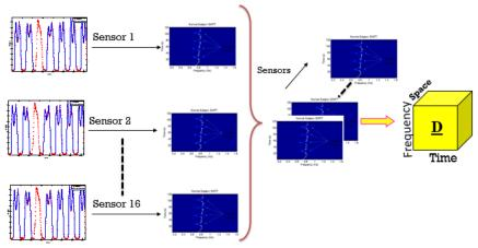
Figure 5.7: PARAFAC Model for the all sensors underneath both feet.
