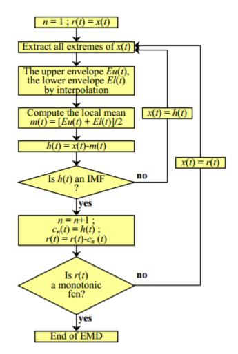
Figure 2.3. Flowchart of Empirical Mode Decomposition algorithm
