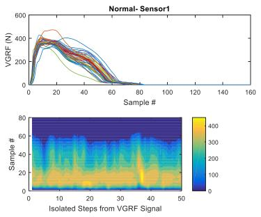
Figure 4.14: Stance phases being isolated from VGRF extracted from the heel sensor underneath the left foot of a normal gait subject and their contour plot
