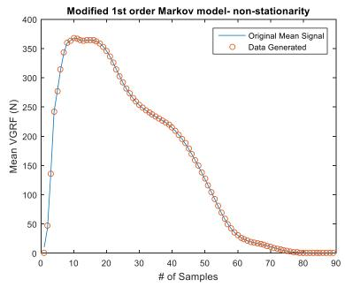
Figure 4.18: Data generated by the modified Markov-Model V.S. Raw Experimental Data An acceptable data modelling as shown in Fig.4.18 is then reached using the new proposed model. The percentage of fitting increased to reach 99.76% on average. This result is generalized to cover all other sensors with variable percent of error but still are highly acceptable. A summary of the algorithm is expressed in Fig.4.19.
