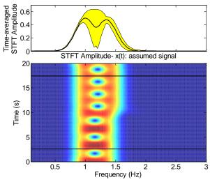
Figure 3.8. STFT and its time averaged applied on the assumed signal x(t)
