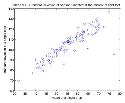
Figure 3.28: Standard deviation versus mean for an abnormal subject upon midsensor located in the right foot.
