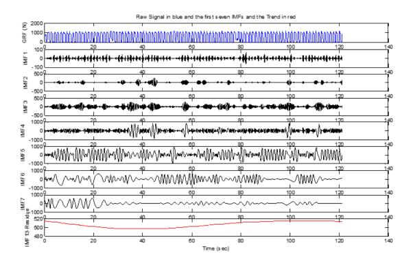
Figure 3.6. The first raw is the original signal. Seven IMFs plus the trend are plotted
