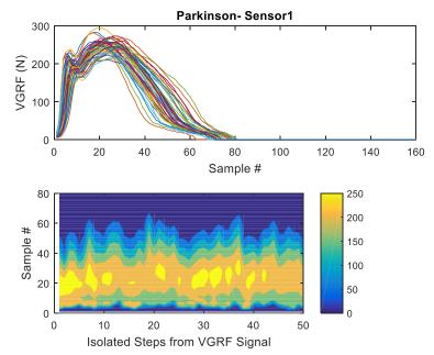
Figure 4.15: Stance phases being isolated from VGRF extracted from the heel sensor underneath the left foot of a Parkinson gait subject and their contour plot
