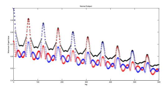
Figure 3.23: Maximum Eigenvalues being computed at different time lags for left sensor to right foot sensors (Red), left sensor to Left foot sensors (Blue), and black indicates when computed for all sensors as one matrix.
