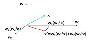
Figure 2.5. Maximizing the variance of the projection in the residual subspace
