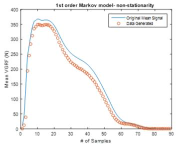
Figure 4.17: Data generated by markov-Model V.S. Raw Experimental Data
