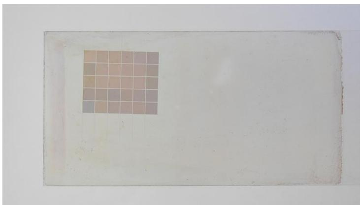
**Figure 3.1: Glass support coated with the  $\text{TiO}_2$  printable material, after been printed several times with different laser settings. Each of the squares in the grid have an area of  $2 \text{ mm} \times 2 \text{ mm}$ .**
