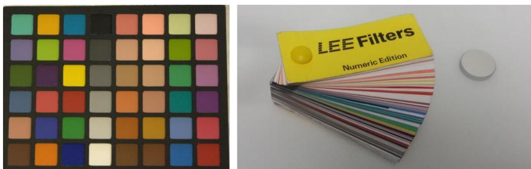
Figure 4.4: Diffuse/matte (left) and specular (right) calibration samples.
