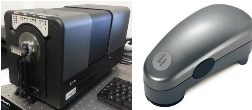
Figure 3.5: X-rite Color i7® (left) X-rite il Pro® (right) spectrophotometers used for reflection and transmission measurements in specific geometries.
