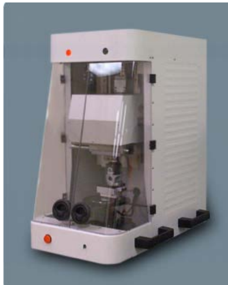
Fig. 6.1 Micotribometrul UMT-2 ( http://www.cetr.com/ )
