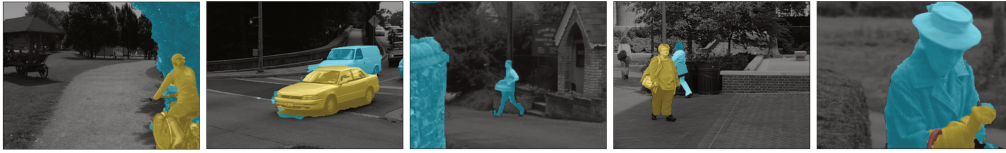
Figure 4.3 – Sample of the segmentation results produced by the method of [134] on FBMS. Grey, blue, yellow and red regions correspond to different scene layers inferred by the method. (Image courtesy of Taylor et al. [134])
