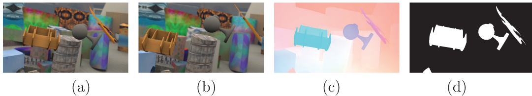
Figure 4.1 – (a,b) Two example frames from a sequence in the FlyingThings3D dataset [97]. The camera is in motion in this scene, along with four independently moving objects. (c) Ground-truth optical flow of (a), which illustrates motion of both foreground objects and background with respect to the next frame (b). (d) Ground-truth segmentation of moving objects in this scene.
