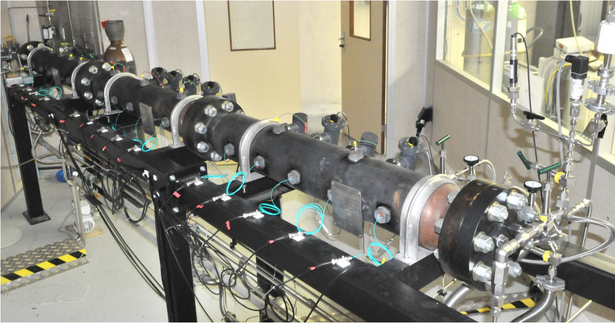
Figure 5.1: Picture of the combustion tube. Here, the device is composed by three sections (TR400, TR200 and TR300).
