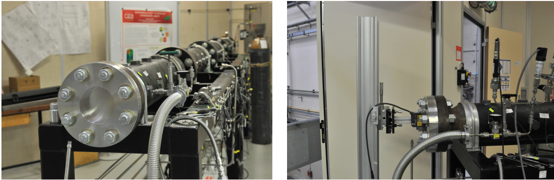
(a) Circular plate clamped between two flanges. (b) Laser support for displacement measurements.
