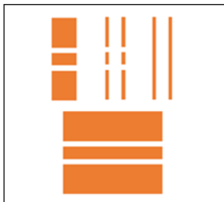
FIGURE III.1 – Standards de calibrage TRL en technologie coplanaire (Respectivement THRU , REFLECT – Open et Short – LINE )
