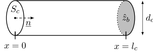
Figure 1.2. Cylindrical impedance tube of length l_c , diameter d_c , cross-section S_c , backing impedance \hat{z}_b , and characteristic impedance z_c .
