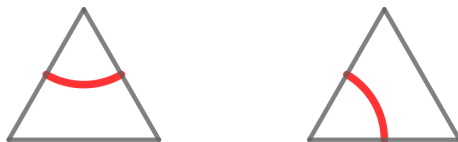
Figure 11: The 2 ways of crossing a triangle for a loop coming from the upper left edge. This rule prevents loops from intersecting each other.
