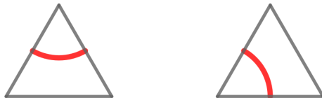
Figure 11: The 2 ways of crossing a triangle for a loop coming from the upper left edge. This rule prevents loops from intersecting each other.
