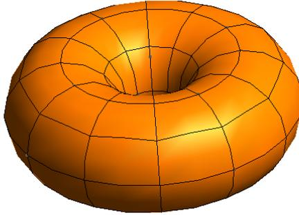
FIGURE 5.1. Computational domain  $\Omega$ . Only the macrocells of the mesh are visible. The represented mesh contains 240 macrocells (poloidal refinement set to  $n_{\text{pol}} = 3$  and toroidal refinement set to  $n_{\text{tor}} = 3$ . In the numerical experiments, we take  $n_{\text{pol}} = 3$  and  $n_{\text{tor}} = 5$ , which leads to a mesh of 400 macrocells). Each macrocell is then cut regularly into the three directions.
