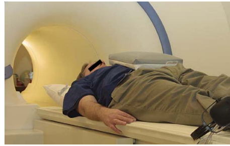
(b) Placement on the abdomen for optimal impact on RF homogeneity, with the white side on the patient. This can however induce B_0 distortions.
