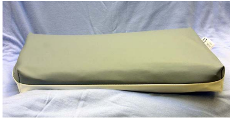
(a) Gel-filled RF cushion; dimensions ( L \times W \times H ): 36 cm \times 26 cm \times 3 cm. Water-based gel mix is located in the white part, while the grey part is a simple foam pad.
