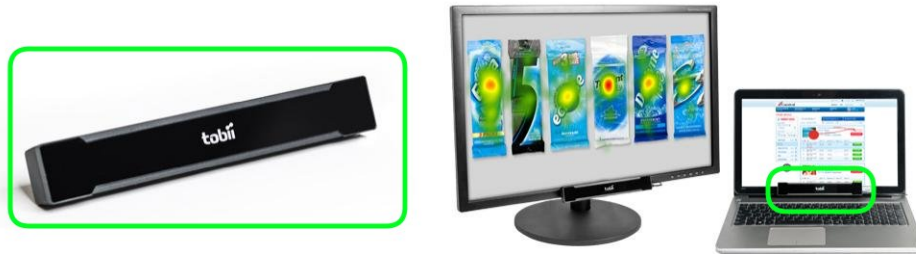
Figure 2.4: Tobii X2-30 eye-tracker appearance.
