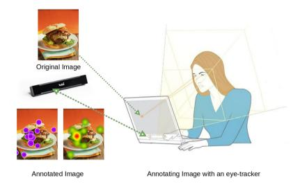
Figure 2.5: The working principle of eye-tracker.
