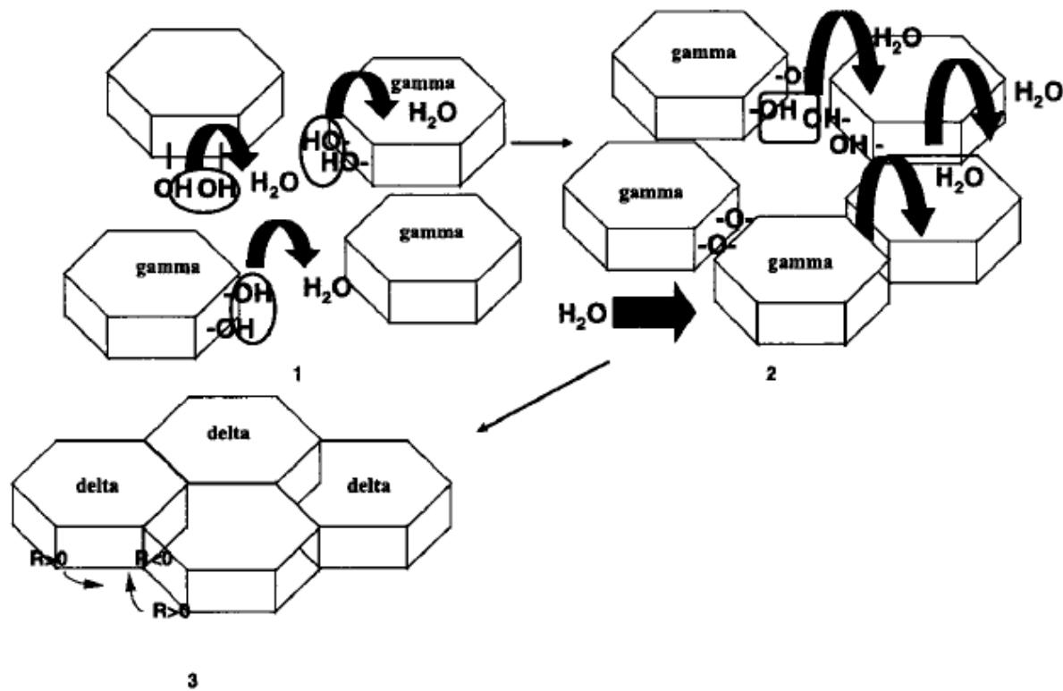
Figure S9. Simplified Scheme of the transition  $\gamma \rightarrow \delta \rightarrow \theta \rightarrow \alpha$ : 1: dehydroxylation of  $\gamma\text{-Al}_2\text{O}_3$  ; 2 : formation of Al-O-Al bridges between platelets ; 3:  $\gamma \rightarrow \delta\text{-Al}_2\text{O}_3$  transition.
