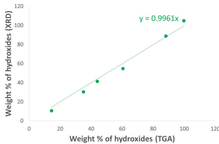
Figure S7. Weight percentage of hydroxide determined by XRD as a function of that determined by TGA for a series of  $\gamma$ -alumina aged at  $70^\circ\text{C}$  in water.
