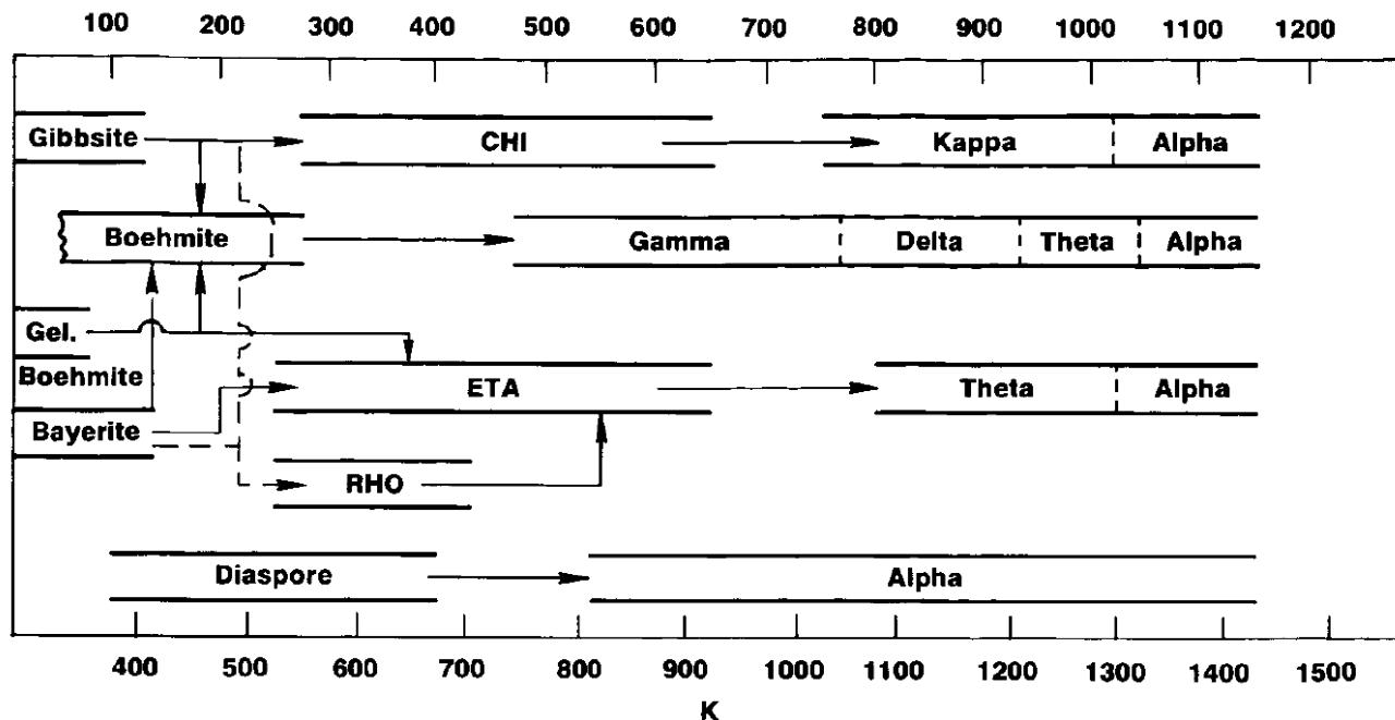
Figure S1. Thermal transformation sequences of transition aluminas. On the left part, aluminum (oxy)hydroxides and on the central and right parts, aluminum oxides.<sup>1</sup>
