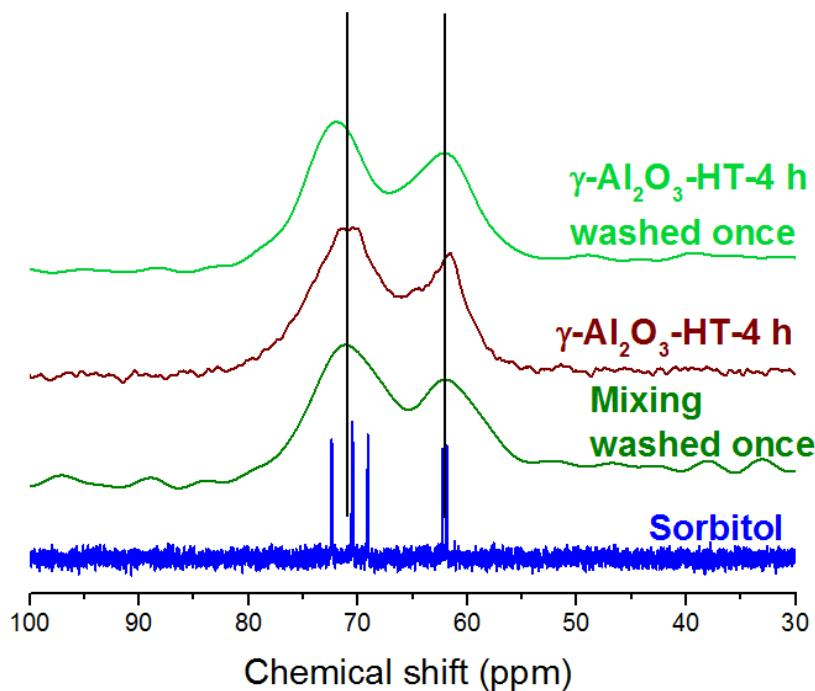
Figure 19.  $^{13}\text{C}$  NMR spectra of sorbitol dissolved in water ( $0.55 \text{ mol.L}^{-1}$ ) (blue), mixing of  $\gamma\text{-Al}_2\text{O}_3$  and sorbitol washed once (green),  $\gamma\text{-Al}_2\text{O}_3$  subjected to an ageing treatment at  $150^\circ\text{C}$  during 4 h under hydrothermal conditions (brown) and washed once (light green).
