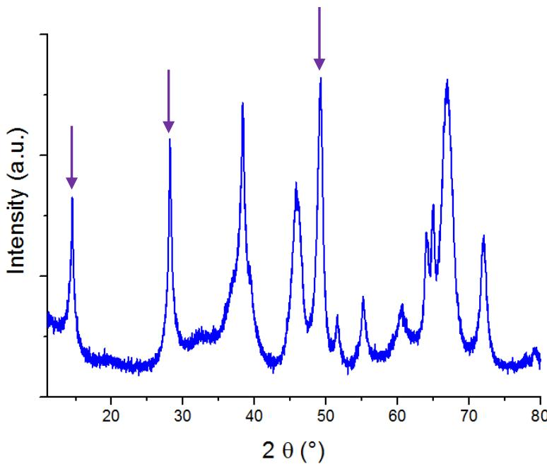
*Figure S1.* XRD pattern of  $\gamma\text{-Al}_2\text{O}_3$  (PDF No. 10-0425) subjected to an ageing treatment in water at  $150^\circ\text{C}$  under hydrothermal conditions during 4 h (1.6g/80 mL).  $\downarrow$  : boehmite peaks used for the calibration method (PDF No. 83-1505).
