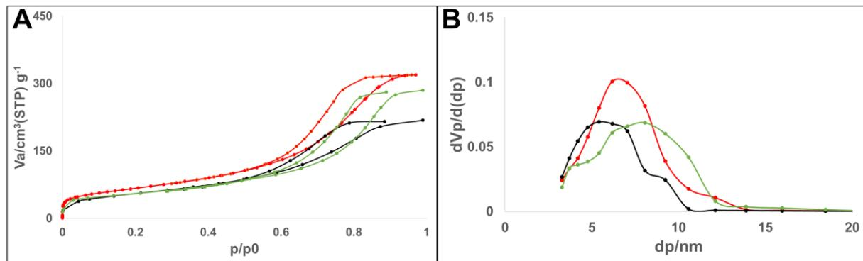
*Figure 18. Adsorption desorption isotherms and BJH plot of  $\gamma\text{-Al}_2\text{O}_3$  (red) and  $\gamma\text{-Al}_2\text{O}_3$  subjected to an ageing treatment in water (green) and with 0.25 mol. $\text{L}^{-1}$  sorbitol (black) at 150°C during 4 h (1.6 g/80 mL, hydrothermal conditions).*
