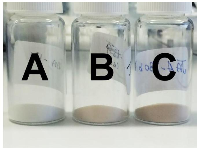
*Figure 17. Photo of  $\gamma\text{-Al}_2\text{O}_3$  samples subjected to an ageing treatment at 150°C under stirring: in presence of water during 4 h (A); in an aqueous solution of 0.25 mol. $\text{L}^{-1}$  sorbitol during 4 h (B) and 14 h (C) (1.6 g/80 mL, hydrothermal conditions).*
