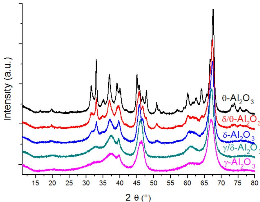
Figure 1. XRD patterns of transition aluminas obtained by calcination of boehmite at: 500°C ( $\gamma$ -Al<sub>2</sub>O<sub>3</sub>, pink, PDF No. 10-0425), 700°C ( $\gamma/\delta$ -Al<sub>2</sub>O<sub>3</sub>, green), 850°C ( $\delta$ -Al<sub>2</sub>O<sub>3</sub>, blue, PDF No. 16-0394), 900°C ( $\delta/\theta$ -Al<sub>2</sub>O<sub>3</sub>, red) and 1000°C ( $\theta$ -Al<sub>2</sub>O<sub>3</sub>, black, PDF No. 23-1009).
