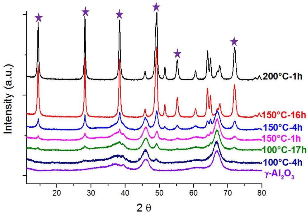
Figure 2. XRD patterns of  $\gamma\text{-Al}_2\text{O}_3$  (purple), subjected to an ageing treatment in water under hydrothermal conditions at different temperatures/ageing times (1.6 g/80 mL). ★ : boehmite (PDF No. 83-1505).
