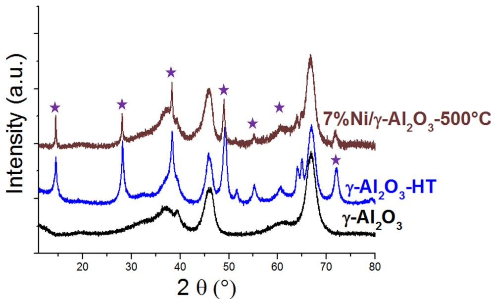
Figure 1. XRD patterns of  $\gamma\text{-Al}_2\text{O}_3$  (black, PDF No. 10-0425) and  $\gamma\text{-Al}_2\text{O}_3\text{-HT}$  (blue) and 7%Ni/ $\gamma\text{-Al}_2\text{O}_3$  (brown) subjected to an ageing treatment in water at 150°C under hydrothermal conditions (HT) during 4 h (1.6 g/80 mL). ★ : boehmite (PDF No. 83-1505).
