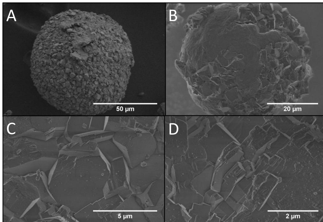
Figure 5. SEM images at different magnifications of  $\gamma$ -Al<sub>2</sub>O<sub>3</sub> subjected to an ageing treatment at 70°C during 7 days (168 h) without stirring (0.6 g/30 mL of distilled water, atm. pressure).
