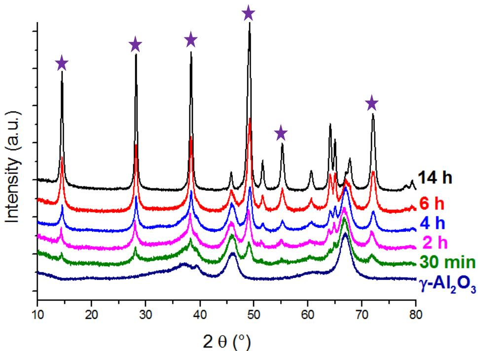
*Figure 8. XRD patterns of  $\gamma\text{-Al}_2\text{O}_3$  (dark blue, PDF No. 10-0425) subjected to an ageing treatment in water at 150°C under hydrothermal conditions during 30 min (green), 2 h (pink), 4 h (blue), 6 h (red) and 14 h (black) (1.6g/80 mL). ★ : boehmite (PDF No. 83-1505).*
