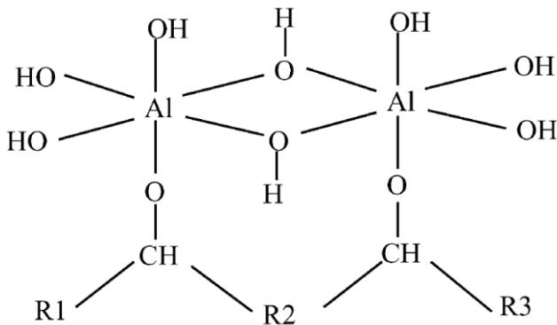
Figure 27. Molecular complex between gibbsite seed and a polyhydroxyl additive.<sup>23</sup>
