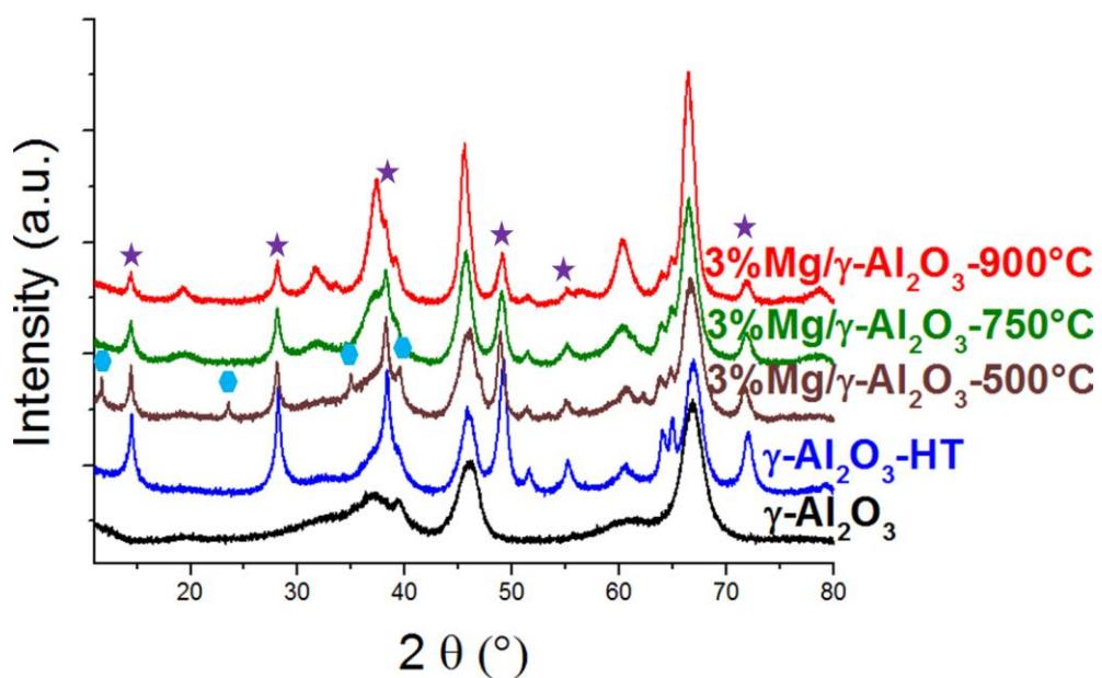
Figure 4. XRD patterns of  $\gamma$ -Al<sub>2</sub>O<sub>3</sub> (black) and  $\gamma$ -Al<sub>2</sub>O<sub>3</sub>-HT (blue) and 3%Mg/ $\gamma$ -Al<sub>2</sub>O<sub>3</sub> calcined at 500°C (brown), 750°C (green) and 900°C (red) and subjected to hydrothermal treatment at 150°C during 4 h (1.6 g/80 mL, hydrothermal conditions) (B). ★ : boehmite (PDF No. 83-1505) and ● : hydrotalcite (PDF No. 89-0460)
