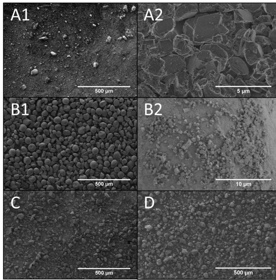
Figure 7. SEM images of  $\gamma$ -Al<sub>2</sub>O<sub>3</sub> subjected to an ageing treatment at 70°C in stirred conditions during 7 days (168 h) in water (A1 and A2 at two different magnifications), 2 h in water (B1 and B2 at two different magnifications), 8 h in water (C) and at 25°C during 5 days in n-heptane (D).
