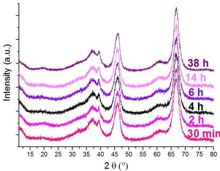
Figure 21. XRD patterns of  $\gamma$ -Al<sub>2</sub>O<sub>3</sub> subjected to an ageing treatment in water with 0.25 mol.L<sup>-1</sup> sorbitol at 150°C during different ageing times up to 38 h (1.6 g/80 mL, hydrothermal conditions).
