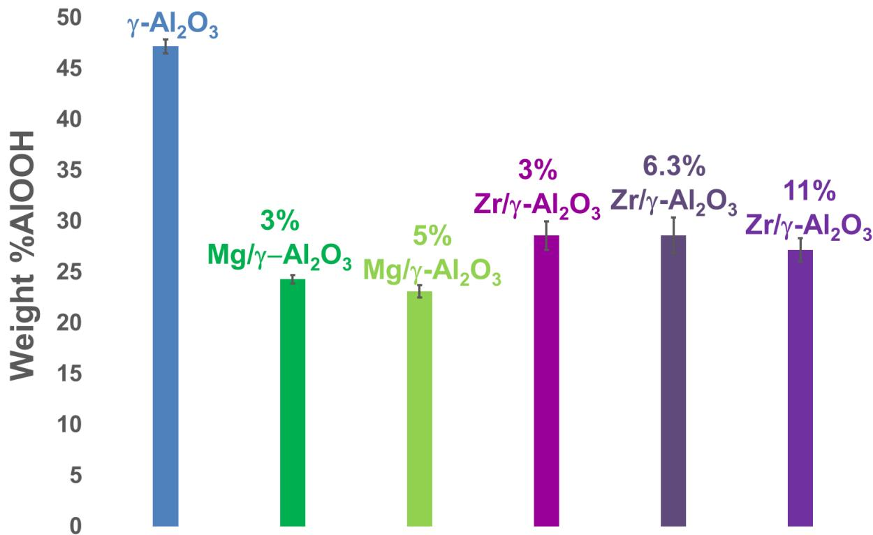
Figure 12. Amount of boehmite formed after ageing  $\gamma\text{-Al}_2\text{O}_3$  in water at 150°C during 4 h after doping with Mg (green) and Zr (purple) and calcination at 500°C, (1.6 g/80 mL, hydrothermal conditions).
