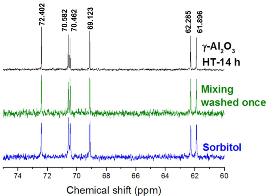
Figure 23.  $^{13}\text{C}$  NMR spectra of sorbitol dissolved in water at a concentration of  $0.55 \text{ mol.L}^{-1}$  (blue), filtrate of a mixing between  $\gamma\text{-Al}_2\text{O}_3$ , sorbitol and water and that was washed once (green) and filtrate of the suspension of  $\gamma\text{-Al}_2\text{O}_3$  subjected to an ageing treatment at  $150^\circ\text{C}$  during 14 h under hydrothermal conditions (black).
