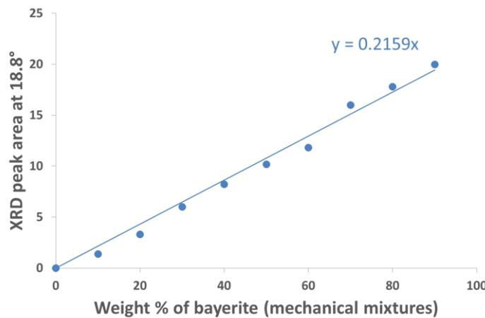
Figure S6. XRD peak intensity at  $2\theta=18.8^\circ$  (bayerite) as a function of the weight % of bayerite in  $\gamma\text{-Al}_2\text{O}_3$ -bayerite mechanical mixtures.
