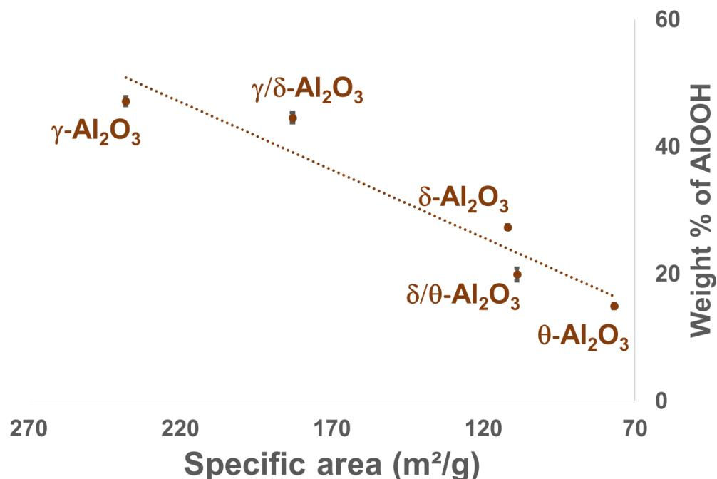
Figure 5. Variation of the total amount of boehmite formed for different transition Al<sub>2</sub>O<sub>3</sub> subjected to an ageing treatment at 150°C during 4 h (1.6 g/80 mL of distilled water, hydrothermal conditions). Quantitative analysis was performed with XRD and TGA.
