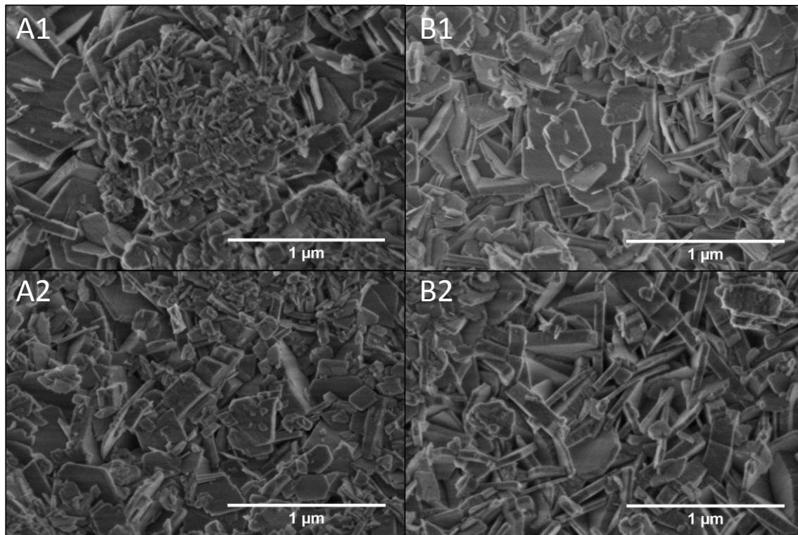
*Figure S7. SEM images of 3%Mg/γ-Al<sub>2</sub>O<sub>3</sub> calcined at 500°C (A series) and at 750°C (B series) subjected to an ageing treatment at 150°C during 4 h (1 series) and 14 h (2 series) under hydrothermal conditions (1.6 g/80 mL).*
