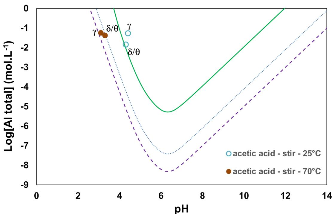
Figure 3. Calculated concentrations of Al(III) in solution (log scale) as a function of pH for  $\gamma\text{-Al}_2\text{O}_3$  (solid green line), bayerite (dotted blue line), and gibbsite (dashed purple line). Experimental data points are shown as empty and filled circles for suspensions of  $\gamma\text{-Al}_2\text{O}_3$  and  $\delta/\theta\text{-Al}_2\text{O}_3$  aged in presence of acetic acid at 25°C and 70°C respectively (0.6 g/30 mL for distilled water, atm. pressure).
