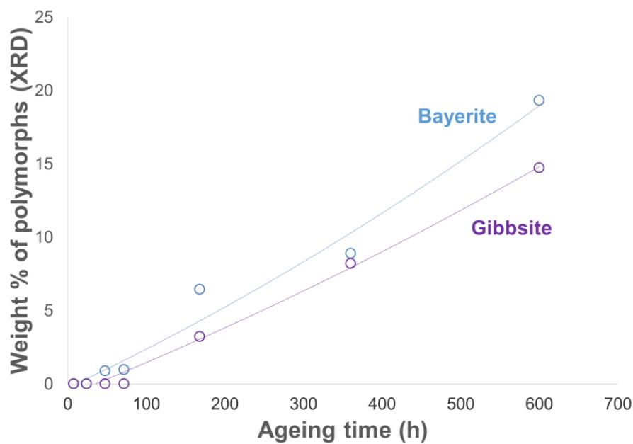
Figure S9. Variation of the amount of bayerite (blue) and gibbsite (purple) after ageing  $\gamma\text{-Al}_2\text{O}_3$  in water under stirring at 25°C (0.6 g/30 mL, atm. pressure).
