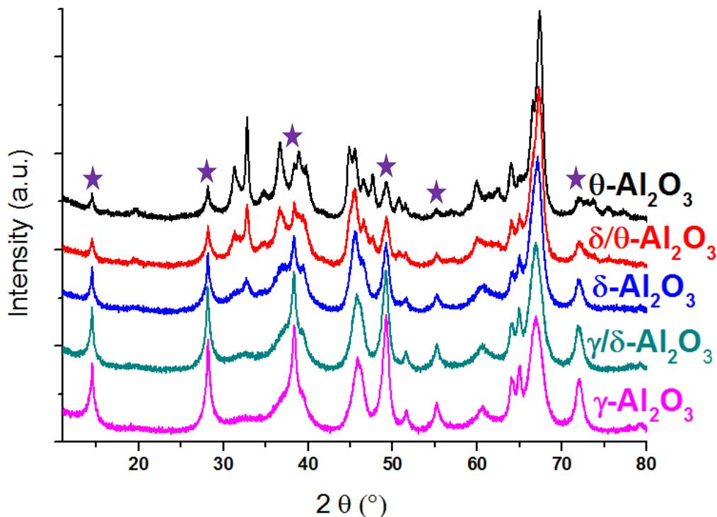
Figure 3. XRD patterns of various alumina polymorphs subjected to an ageing treatment in water at 150°C under stirring during 4 h (1.6 g/80 mL, hydrothermal conditions) :  $\gamma\text{-Al}_2\text{O}_3$  (pink),  $\gamma/\delta\text{-Al}_2\text{O}_3$  (green),  $\delta\text{-Al}_2\text{O}_3$  (blue),  $\delta/\theta\text{-Al}_2\text{O}_3$  (red) and  $\theta\text{-Al}_2\text{O}_3$  (black) ★ : boehmite (PDF No. 83-1505).
