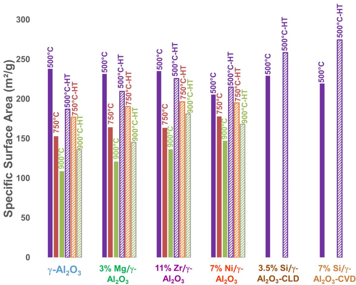
Figure 6. Specific surface areas of  $\gamma\text{-Al}_2\text{O}_3$ , 3%Mg/ $\gamma\text{-Al}_2\text{O}_3$ , 11%Zr/ $\gamma\text{-Al}_2\text{O}_3$ ; 7%Ni/ $\gamma\text{-Al}_2\text{O}_3$ , 3.5%Si/ $\gamma\text{-Al}_2\text{O}_3$ -CLD and 7%Si/ $\gamma\text{-Al}_2\text{O}_3$ -CVD calcined at 500°C (purple), 750°C (red) and 900°C (green) and subjected to a hydrothermal treatment (HT, hatched histograms) at 150°C during 4 (1.6 g/80 mL).
