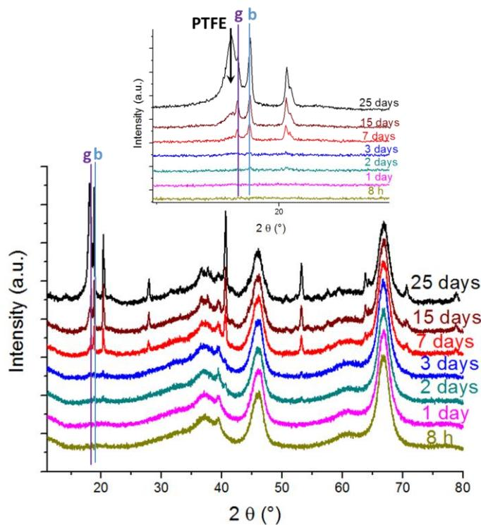
Figure S4. XRD patterns of  $\gamma\text{-Al}_2\text{O}_3$  subjected to an ageing treatment in water at 25°C under magnetic stirring during 8 h (gold), 1 day (pink), 2 days (green), 3 days (blue) and 7 days (red) (0.6 g/30 mL). g: gibbsite (PDF No. 33-18) and b: bayerite (PDF No. 20-11).
