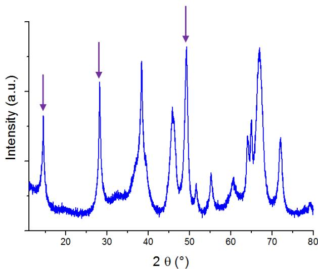
Figure 29. XRD pattern of  $\gamma\text{-Al}_2\text{O}_3$  (PDF No. 10-0425) subjected to an ageing treatment in water at  $150^\circ\text{C}$  under hydrothermal conditions during 4 h (blue) ( $1.6\text{ g}/80\text{ mL}$ ).  $\downarrow$ : boehmite peaks used for the calibration method (PDF No. 83-1505).
