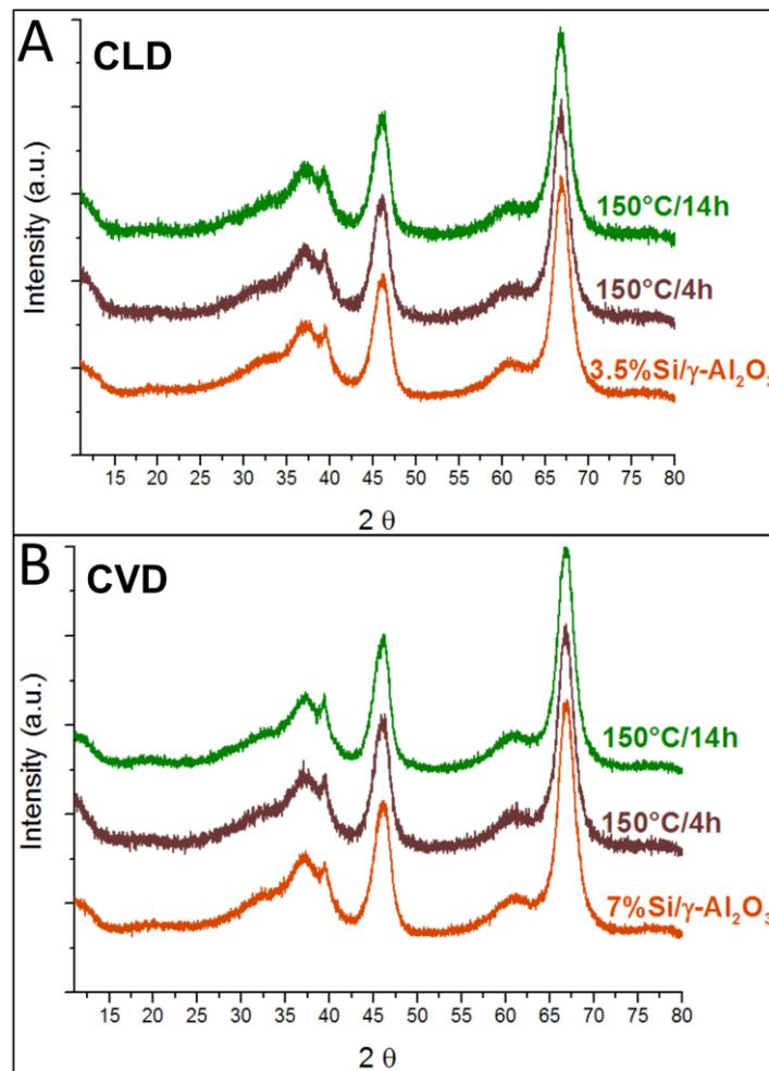
*Figure 2. XRD patterns of 3.5%Si/γ-Al<sub>2</sub>O<sub>3</sub>-CLD and 7%Si/γ-Al<sub>2</sub>O<sub>3</sub>-CVD (orange) subjected to an ageing treatment at 150°C during 4 h (brown) and 14 h (green) (1.6 g/80 mL, hydrothermal conditions).*
