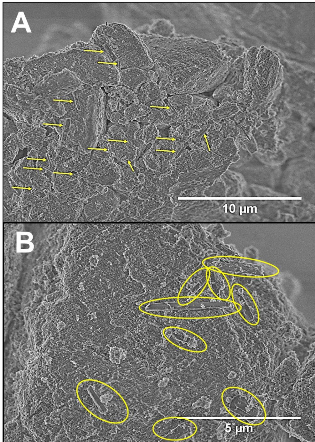
Figure 4. SEM images of  $\gamma$ - $\text{Al}_2\text{O}_3$  subjected to ageing treatment at  $70^\circ\text{C}$  during 7 days in presence of acetic acid. The pH of the suspensions was adjusted and the total weight percentage of the acid relative to the amount of water was 37% (0.6 g / 30 mL, atm. pressure).
