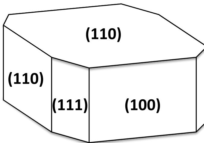
Figure 10.  $\gamma$ -alumina nanoparticle with the corresponding surface orientations.<sup>[63]</sup>
