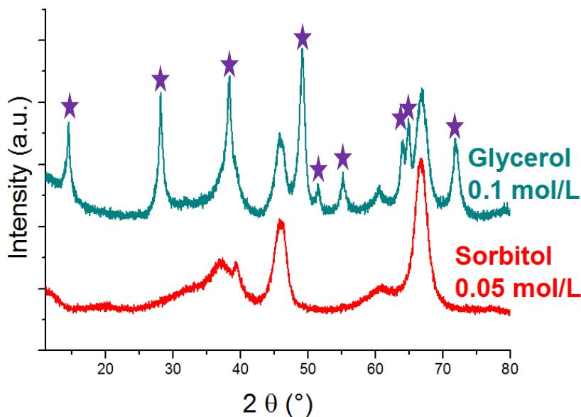
Figure 16. XRD patterns of  $\gamma$ - $\text{Al}_2\text{O}_3$  subjected to an ageing treatment at  $150^\circ\text{C}$  under stirring during 4 h in an aqueous solution of  $0.05 \text{ mol.L}^{-1}$  sorbitol (red) or  $0.1 \text{ mol.L}^{-1}$  glycerol (light blue) ( $1.6 \text{ g}/80 \text{ mL}$ , hydrothermal conditions). ★ : boehmite (PDF No. 83-1505).
