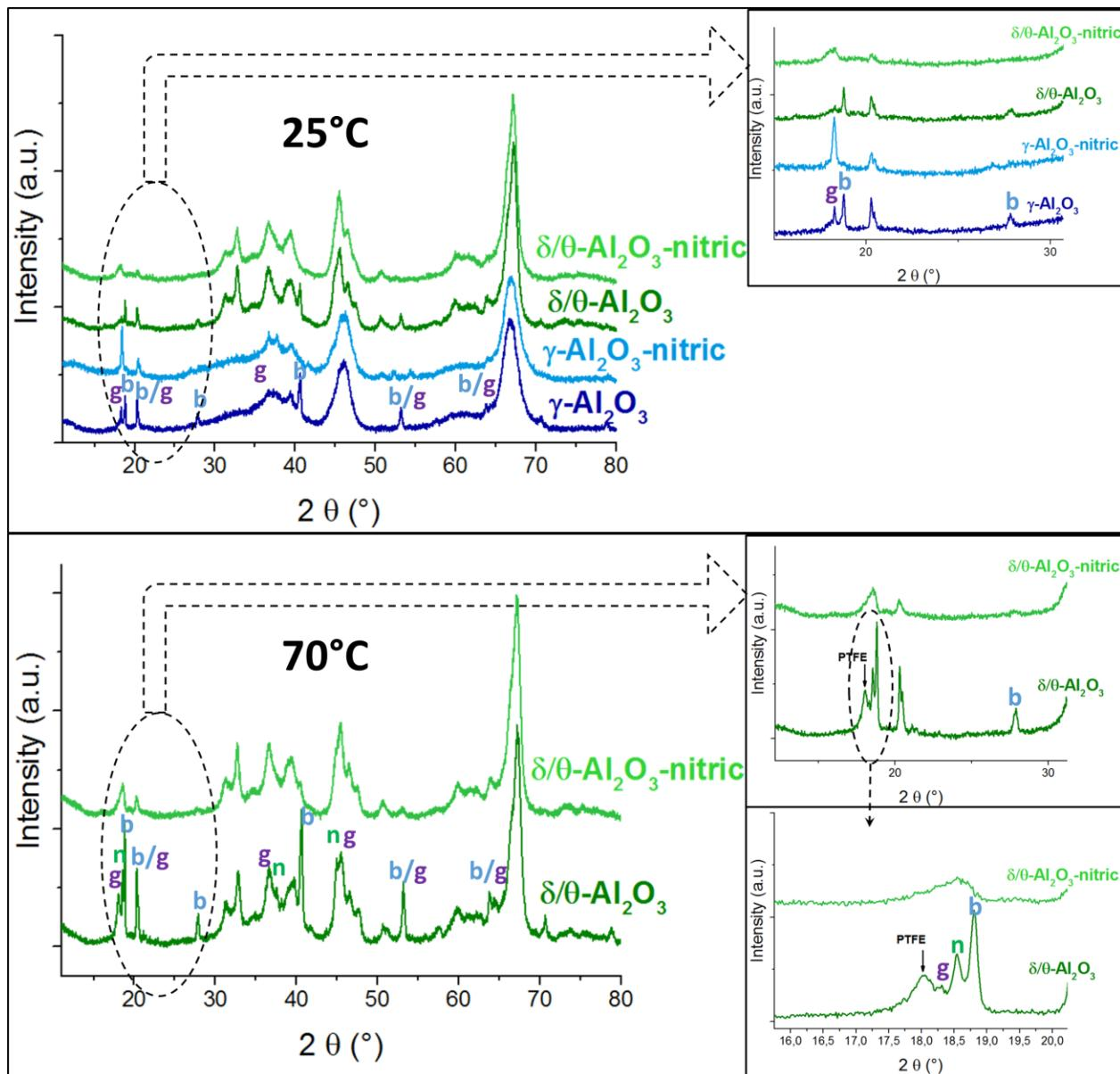
Figure 1. XRD patterns of  $\gamma\text{-Al}_2\text{O}_3$  (blue) and  $\delta/\theta\text{-Al}_2\text{O}_3$  (green) subjected to ageing treatment at 25°C during 11 days (A) and 70°C during 7 days (B) in water only (dark blue and dark green) and with nitric acid (light blue and light green). The pH of the suspensions was adjusted to 3. g: gibbsite, n: nordstrandite and b: bayerite. (0.6 g / 30 mL, atm. pressure).
