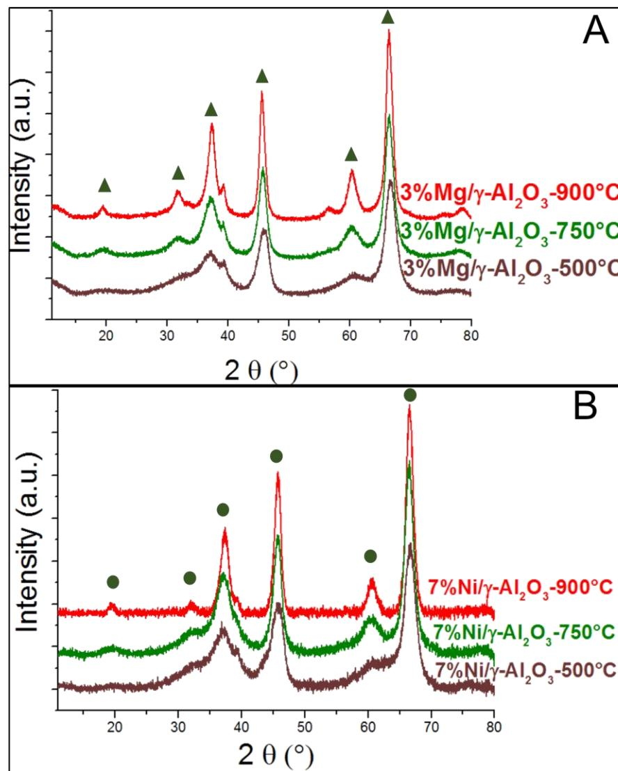
Figure 3. XRD patterns of  $\gamma\text{-Al}_2\text{O}_3$  doped by Mg<sup>II</sup> (A) and Ni<sup>II</sup> (B) and calcined at 500°C, 750°C and 900°C. ▲: MgAl<sub>2</sub>O<sub>4</sub> (PDF No. 87-0340), ●: NiAl<sub>2</sub>O<sub>4</sub> (PDF No. 10-0339).
