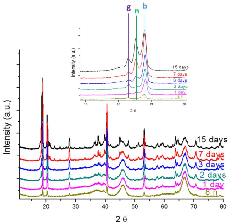
Figure S5. XRD patterns of  $\gamma$ -Al<sub>2</sub>O<sub>3</sub> subjected to an ageing treatment in water at 70°C under magnetic stirring during 8 h (gold), 1 day (pink), 2 days (green), 3 days (blue), 7 days (red) and 15 days (black) (0.6 g/30 mL).
