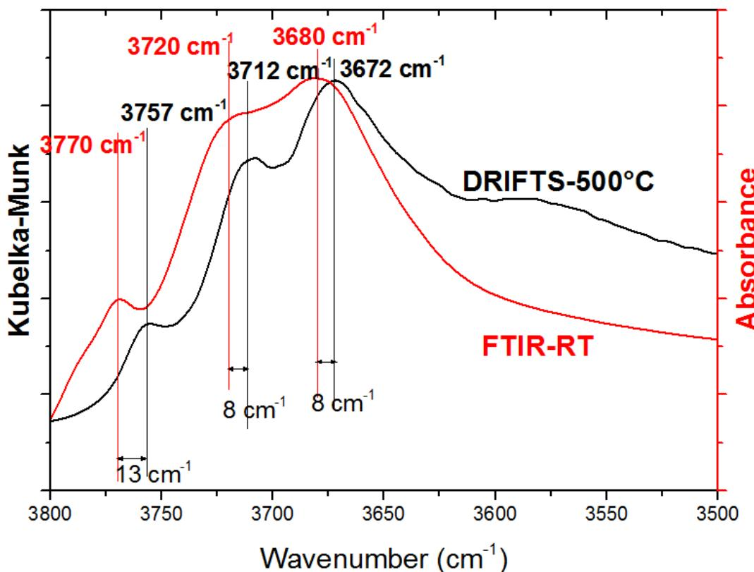
*Figure S10. Infrared spectra of  $\gamma\text{-Al}_2\text{O}_3$  in the  $\nu_{\text{OH}}$  region: in black, spectrum recorded in the diffuse reflectance mode (DRIFTS) at 500°C; in red spectrum recorded in the transmission mode (FTIR) at room temperature.*
