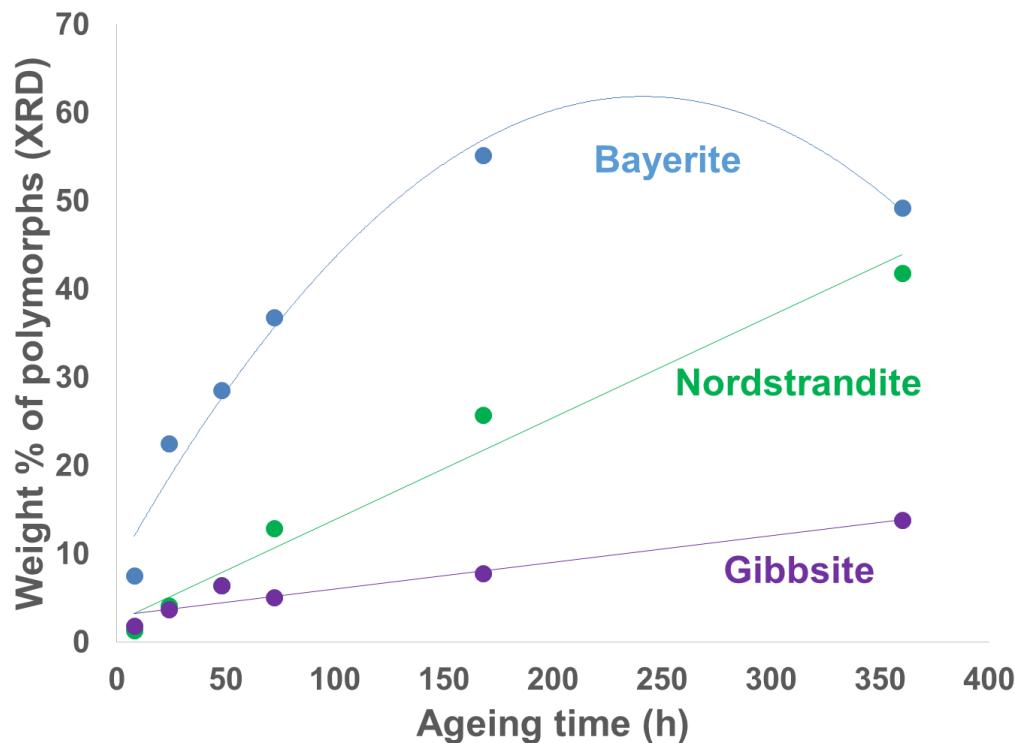
Figure 9. Variation of the amount of bayerite (blue), nordstrandite (green) and gibbsite (purple) after ageing  $\gamma\text{-Al}_2\text{O}_3$  in water under stirring at 70°C (0.6 g/30 mL, atm. pressure).
