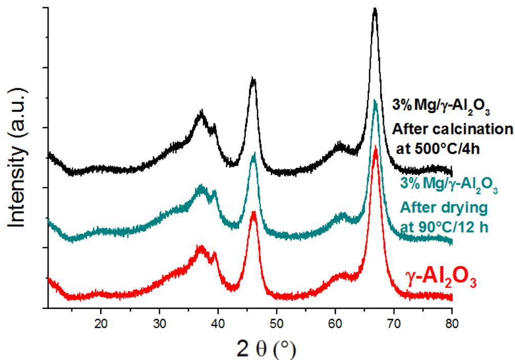
Figure S6. XRD patterns of  $\gamma$ -Al<sub>2</sub>O<sub>3</sub> (red) and 3%Mg/ $\gamma$ -Al<sub>2</sub>O<sub>3</sub> after impregnation of Mg and drying at 90°C during 12 h (cyan) and after calcination at 500°C during 4 h (black).
