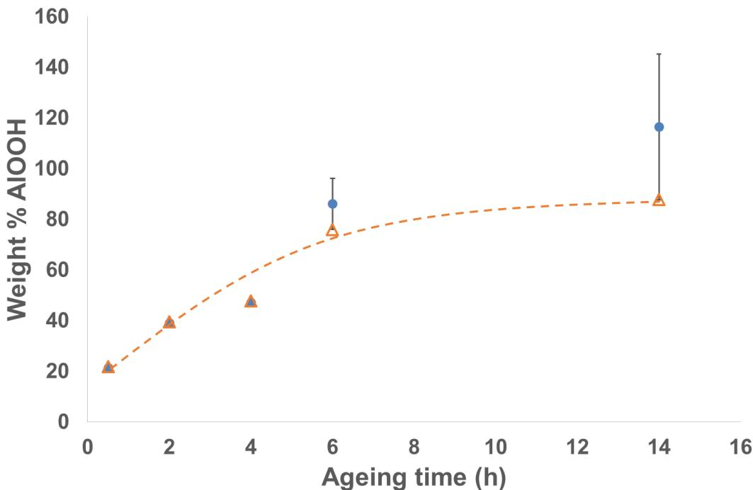
*Figure 9. Variation of the amount of boehmite formed after ageing  $\gamma\text{-Al}_2\text{O}_3$  in water for different times under stirring at 150°C (1.6 g/80 mL, hydrothermal conditions). Triangles correspond to the TGA analyses. Circles are the average of the XRD and TGA analyses and error bars are the standard deviation between both methods (see in the text).*
