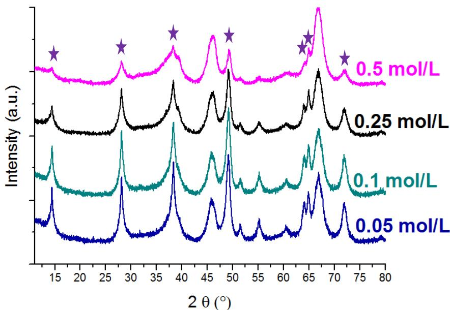
Figure 26. XRD patterns of  $\gamma\text{-Al}_2\text{O}_3$  subjected to an ageing treatment in water with different concentrations of glycerol at 150°C during 4 h (1.6 g/80 mL, hydrothermal conditions). ★ : boehmite (PDF No. 83-1505).
