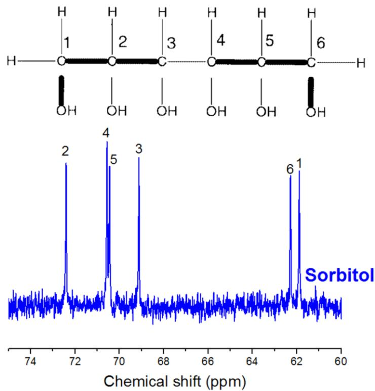
*Figure 20. Chemical structure of sorbitol and numbering of their carbons in the Fischer representation.<sup>20</sup>  $^{13}\text{C}$  NMR spectrum of sorbitol dissolved in water ( $0.55 \text{ mol.L}^{-1}$ ).*
