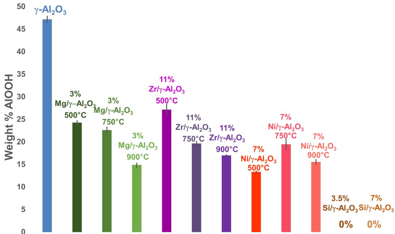
Figure 2. Weight percentage of boehmite formed after ageing  $\gamma\text{-Al}_2\text{O}_3$  doped with 3% Mg (green), 11% Zr (purple), 7% Ni (red) and (3.7 or 7%) Si (brown) in water at 150°C during 4 h (1.6 g/80 mL, hydrothermal conditions). 500°C, 750°C and 900°C refer to the calcination temperature of each doped supports.
