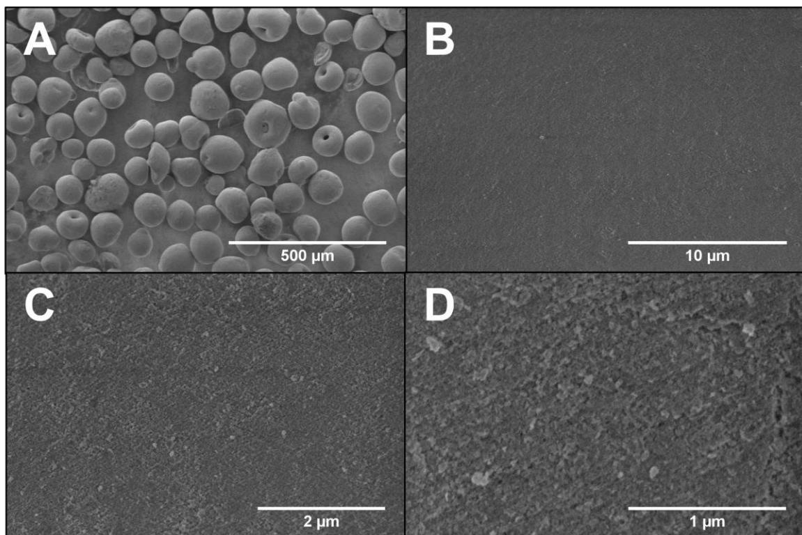
Figure 15. SEM images at different magnifications of  $\gamma$ -Al<sub>2</sub>O<sub>3</sub> subjected to an ageing treatment at 150°C during 4 h in water with 0.25 mol.L<sup>-1</sup> **sorbitol**. (1.6 g/80 mL, hydrothermal conditions).
