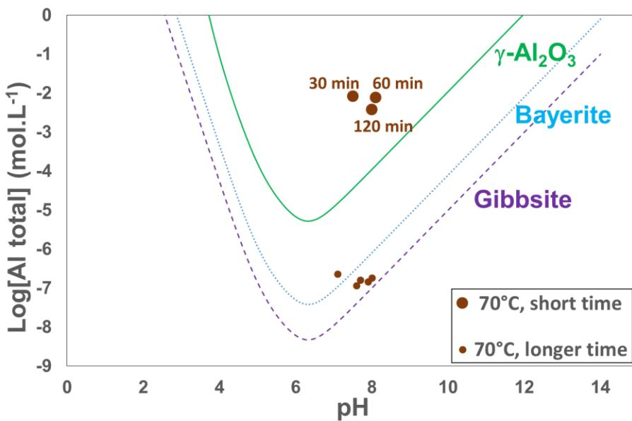
Figure 4. Calculated concentrations of Al(III) in solution (log scale) as a function of pH for  $\gamma\text{-Al}_2\text{O}_3$  (solid green line), bayerite (dotted blue line), and gibbsite (dashed purple line). Experimental data points are shown as filled circles for suspensions aged at 70°C (short time  $\leq 2$  h, longer time  $\geq 8$  h) (0.6 g/30 mL for distilled water, atm. pressure).
