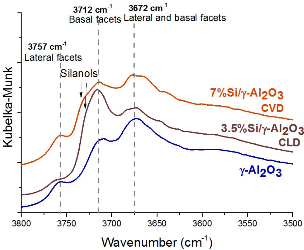
Figure 11. DRIFTS spectra recorded at 500°C of  $\gamma\text{-Al}_2\text{O}_3$  (blue) and 3.5%Si/ $\gamma\text{-Al}_2\text{O}_3$ -CLD (dark brown) and 7%Si/ $\gamma\text{-Al}_2\text{O}_3$ -CVD (light brown).
