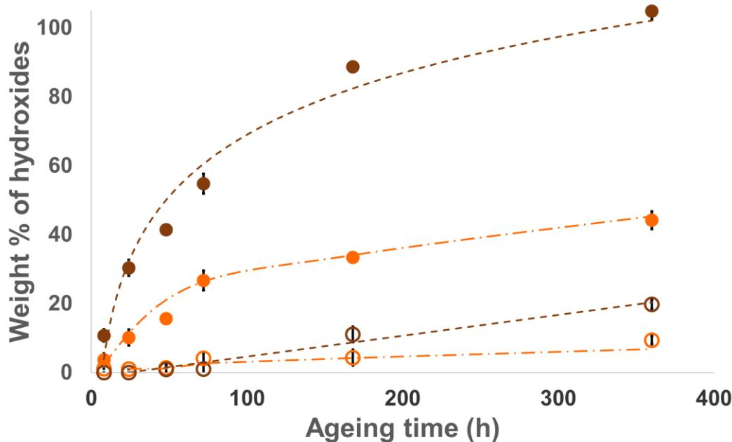
Figure 8. Variation of the amount of hydroxides formed after ageing  $\gamma\text{-Al}_2\text{O}_3$  (brown) and  $\delta/\theta\text{-Al}_2\text{O}_3$  (orange) in water under stirring at 70°C (filled circles) and 25°C (open circles) (0.6 g/30 mL, atm. pressure).
