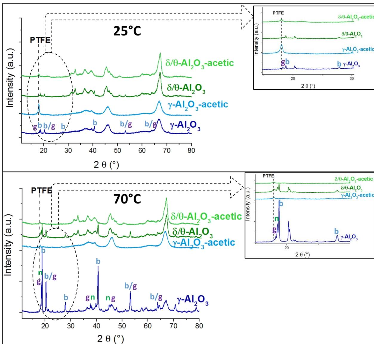
Figure 2. XRD patterns of  $\gamma\text{-Al}_2\text{O}_3$  (blue) and  $\delta/\theta\text{-Al}_2\text{O}_3$  (green) subjected to ageing treatment at 25°C during 11 days (A) and 70°C during 7 days (B) in water only (dark blue and dark green) and with acetic acid (light blue and light green). The pH of the suspensions was adjusted to 3. g: gibbsite, n: nordstrandite and b: bayerite. (0.6 g / 30 mL, atm. pressure).
