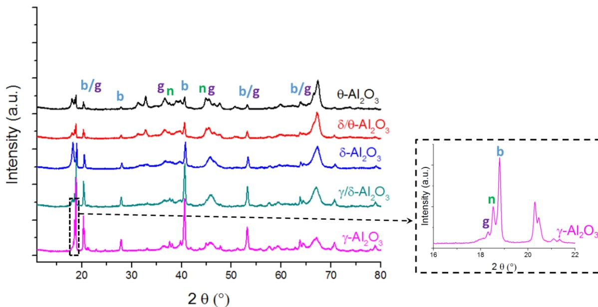
Figure 2. XRD patterns of  $\gamma$ -Al<sub>2</sub>O<sub>3</sub> (pink),  $\gamma/\delta$ -Al<sub>2</sub>O<sub>3</sub> (green),  $\delta$ -Al<sub>2</sub>O<sub>3</sub> (blue),  $\delta/\theta$ -Al<sub>2</sub>O<sub>3</sub> (red) and  $\theta$ -Al<sub>2</sub>O<sub>3</sub> (black) subjected to an ageing treatment in water at 70°C under stirring during 7 days (168 h) (0.6g/30 mL). g: gibbsite (PDF No. 33-18), n: nordstrandite (PDF No. 85-1049) and b: bayerite (PDF No. 20-11).
