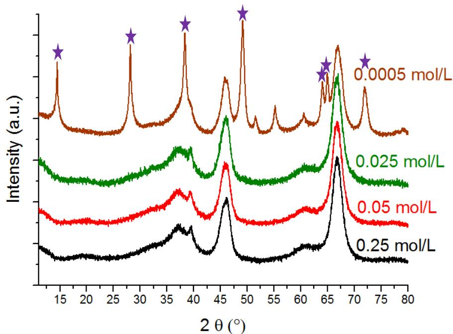
*Figure 24. XRD patterns of  $\gamma\text{-Al}_2\text{O}_3$  subjected to an ageing treatment in water with different concentrations of sorbitol at  $150^\circ\text{C}$  during 4 h (1.6 g/80 mL, hydrothermal conditions). ★ : boehmite (PDF No. 83-1505).*
