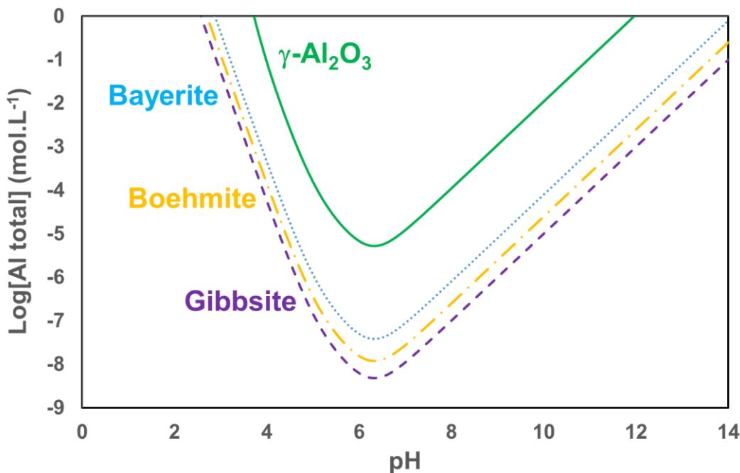
Figure 4. Calculated concentrations of Al[III] in solution (log scale) as a function of pH for  $\gamma\text{-Al}_2\text{O}_3$  (solid green line), bayerite (dotted blue line), boehmite (dash-dotted yellow line) and gibbsite (dashed purple line).
