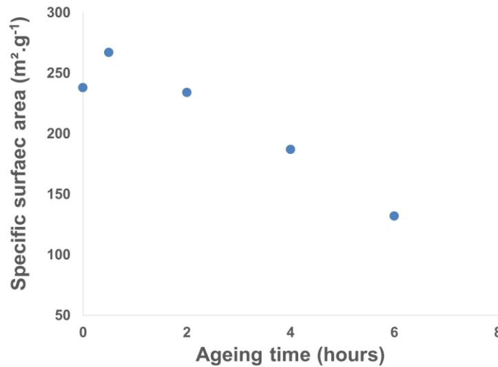
*Figure 11. Variation of the specific surface area of  $\gamma\text{-Al}_2\text{O}_3$  subjected to an ageing treatment at 150°C during different ageing times (1.6 g/80 mL, hydrothermal conditions).*
