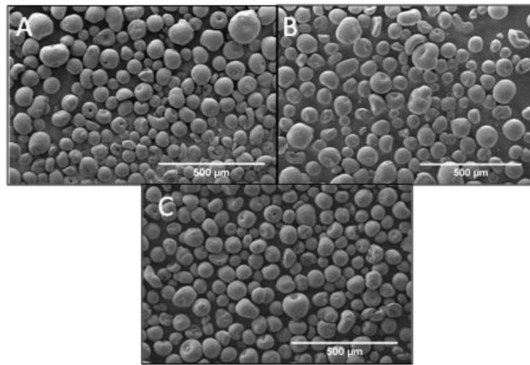
Figure S2. SEM images of: (A) boehmite Sasol Pural SB3, (B)  $\gamma$ - $\text{Al}_2\text{O}_3$  obtained by calcining the Pural SB3 at 500°C during 12 h and (C)  $\delta/\theta$ - $\text{Al}_2\text{O}_3$  obtained by calcining the Pural SB3 at 900°C during 12 h.
