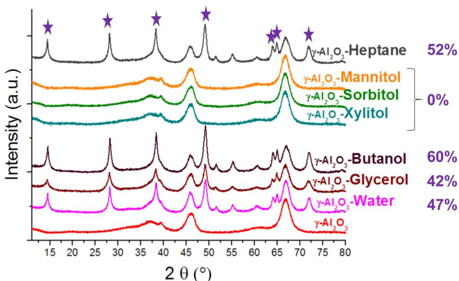
Figure 13. XRD patterns of  $\gamma\text{-Al}_2\text{O}_3$  (red) subjected to an ageing treatment under hydrothermal conditions at  $150^\circ\text{C}$  under stirring during 4 h in presence of water (pink) and  $0.25 \text{ mol.L}^{-1}$  glycerol (bordeaux), butanol (dark purple), xylitol (light blue), sorbitol (green), mannitol (orange) and heptane (dark grey) ( $1.6 \text{ g}/80 \text{ mL}$ ). ★ : boehmite (PDF No. 83-1505). The percentages indicate the amount of boehmite formed.
