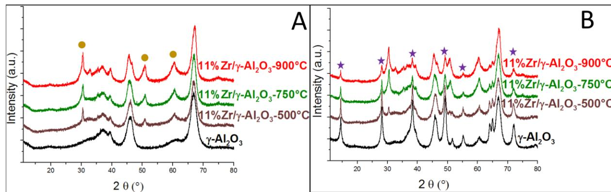
*Figure S8. XRD patterns of (A)  $\gamma\text{-Al}_2\text{O}_3$  (black) and 11% Zr/ $\gamma\text{-Al}_2\text{O}_3$  calcined at 500°C (brown), 750°C (green,) and 900°C (red) and (B) after ageing at 150°C during 4 h (1.6 g/80 mL). ●  $\text{ZrO}_2$  (PDF No 37-1413) ★ : boehmite (PDF No. 83-1505).*
