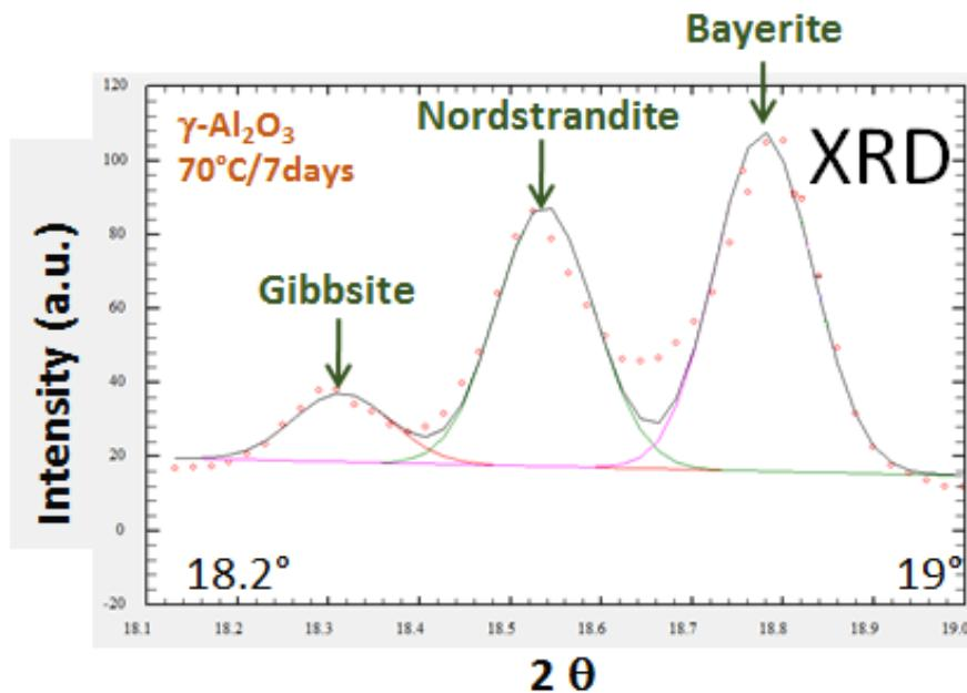
Figure S8. Fitting of the XRD peaks corresponding to hydroxide polymorphs: gibbsite, nordstrandite and bayerite formed after ageing  $\gamma\text{-Al}_2\text{O}_3$  in water at 70°C during 7 days (0.6 g/30 mL, atm. pressure).
