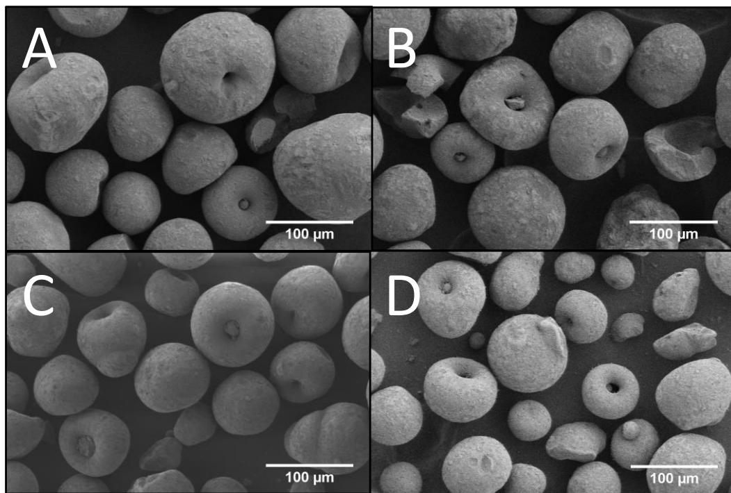
Figure 6. SEM images of  $\gamma\text{-Al}_2\text{O}_3$  subjected to an ageing treatment at 150°C during 30 min (A), 2 h (B), 4 h (C) and 6 h (D).
