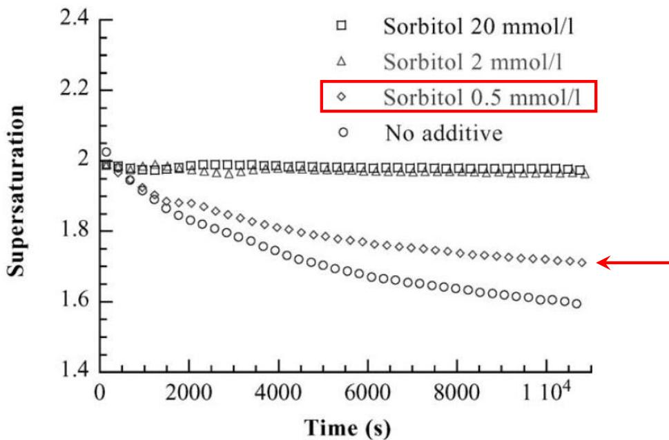
*Figure 25. Effect of sorbitol concentration on gibbsite agglomeration. The term of agglomeration was explained by the authors as the mechanism by which particles existing in a suspension are linked by simultaneous aggregation and growth. It is a phenomenon that happens during the crystallization of gibbsite (a step of the Bayer process). The supersaturation is the concentration of aluminate ions and is measured by means of a conductivity regulation.<sup>23</sup>*
