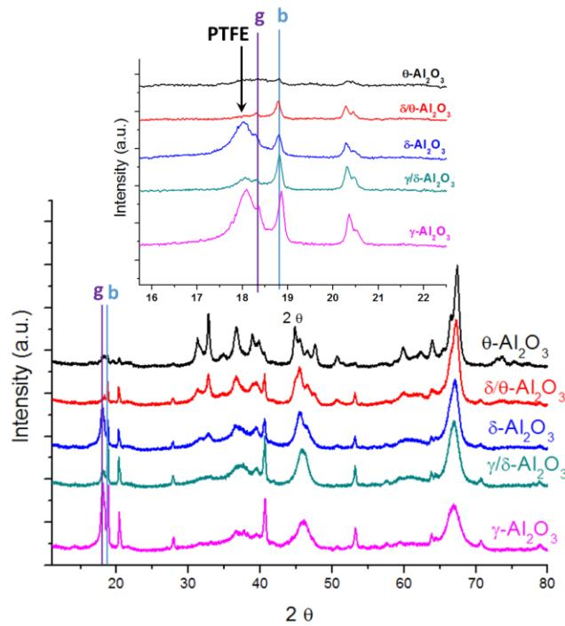
Figure S3. XRD patterns of  $\gamma$ - $\text{Al}_2\text{O}_3$  (pink),  $\gamma/\delta$ - $\text{Al}_2\text{O}_3$  (green),  $\delta$ - $\text{Al}_2\text{O}_3$  (blue),  $\delta/\theta$ - $\text{Al}_2\text{O}_3$  (red) and  $\theta$ - $\text{Al}_2\text{O}_3$  (black) subjected to an ageing treatment in water at 25°C under magnetic stirring during 25 days (600 h) (0.6 g/30 mL). g: gibbsite (PDF No. 33-18) and b: bayerite (PDF No. 20-11).
