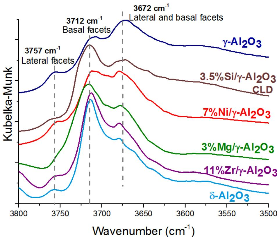
Figure 9. DRIFTS spectra **recorded at 500°C** of  $\gamma\text{-Al}_2\text{O}_3$  (blue), 3.5%Si/ $\gamma\text{-Al}_2\text{O}_3$ -CLD (dark brown), 7%Ni/ $\gamma\text{-Al}_2\text{O}_3$ -500°C (red), 3%Mg/ $\gamma\text{-Al}_2\text{O}_3$ -500°C (green), 11%Zr/ $\gamma\text{-Al}_2\text{O}_3$ -500°C (purple) and  $\delta\text{-Al}_2\text{O}_3$  (light blue).
