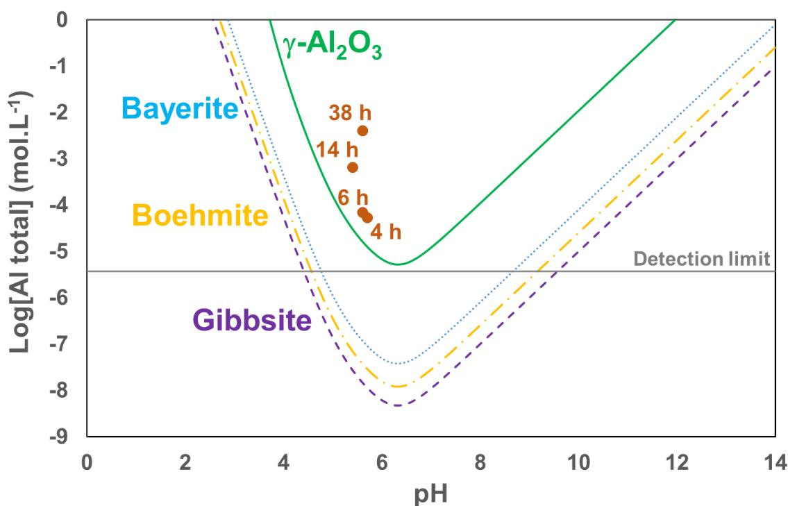
*Figure 22. Concentrations of Al(III) in solution (log scale) as a function of pH for  $\gamma\text{-Al}_2\text{O}_3$  (solid green line), bayerite (dotted blue line), boehmite (dash-dotted yellow line) and gibbsite (dashed purple line). Experimental data points are shown as filled circles for suspensions aged at 150°C in water with 0.25 mol.L<sup>-1</sup> sorbitol during different ageing times up to 38 h (1.6 g/80 mL, hydrothermal conditions).*
