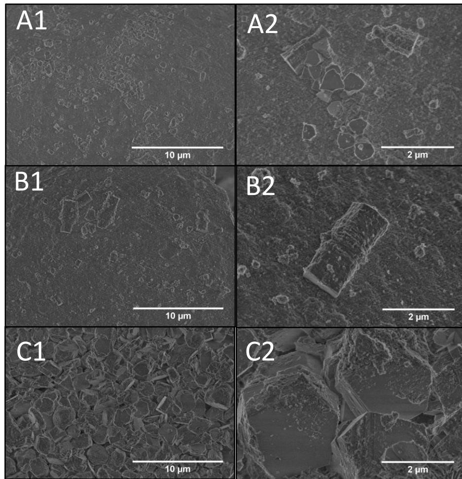
Figure 6. SEM images at different magnifications (series 1 and 2) of  $\gamma\text{-Al}_2\text{O}_3$  subjected to an ageing treatment under stirring at 70°C during 2 h (series A), 8h (series B) and 7 days (168 h) (series C).
