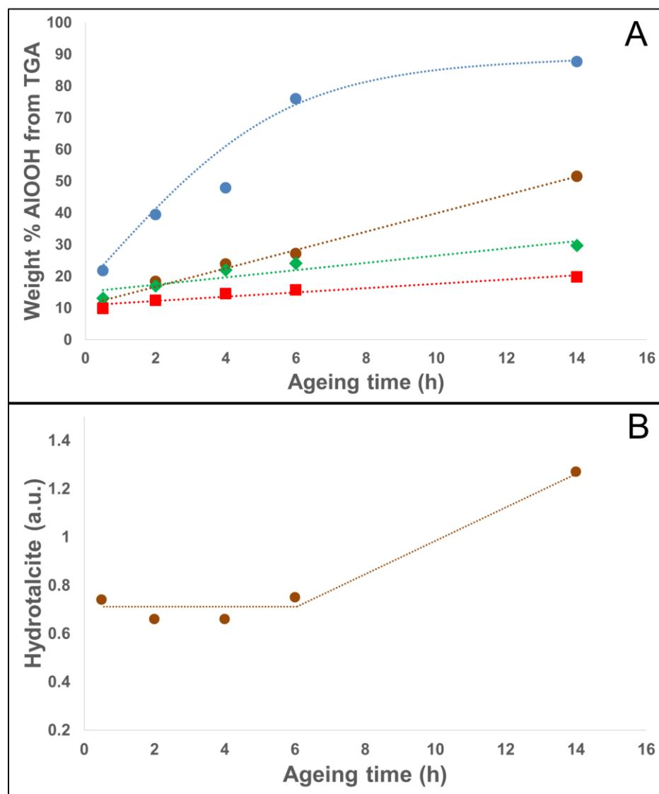
Figure 5. (A) Amount of boehmite formed after ageing  $\gamma$ -Al<sub>2</sub>O<sub>3</sub> (blue circles), 3%Mg/ $\gamma$ -Al<sub>2</sub>O<sub>3</sub>-500°C (brown circles), 3%Mg/ $\gamma$ -Al<sub>2</sub>O<sub>3</sub>-750°C (green diamonds) and 3%Mg/ $\gamma$ -Al<sub>2</sub>O<sub>3</sub>-900°C (red squares) in water at 150°C during different ageing times (1.6 g/80 mL, hydrothermal conditions).
