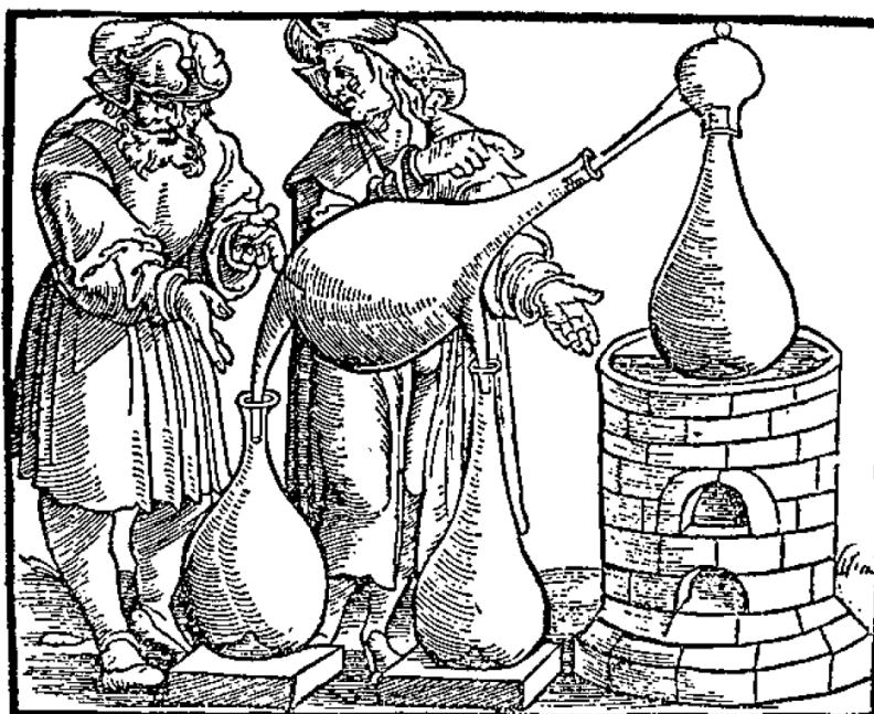
Apparatus for fractionated distillation. Abu Musa Jabir VIII th century. Reedited from Philosophi ac Alchimistae Maximi by Johannes Greininger, Strasbourg, 1531.
