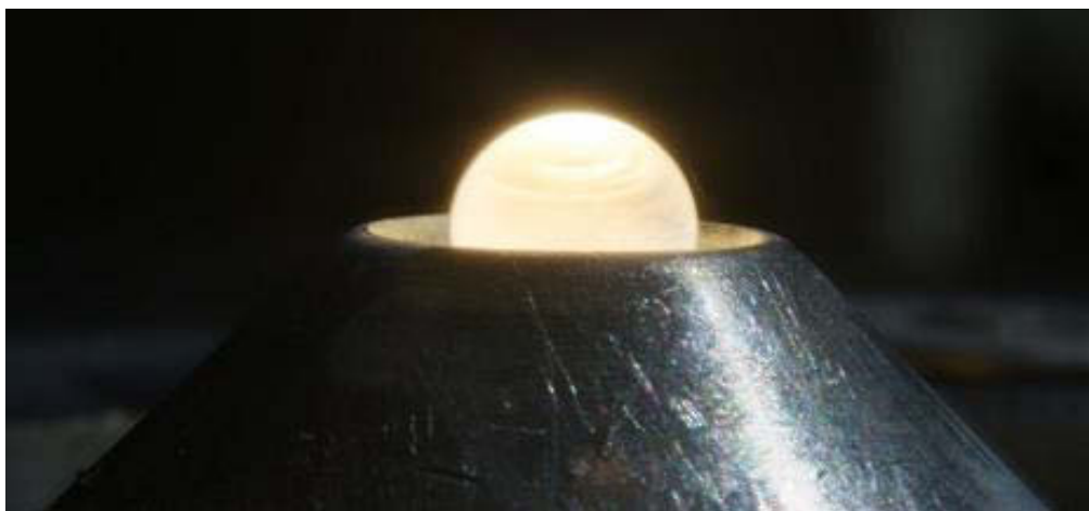
Figure 2.1. Close-up of the molten glass sphere levitating on the aluminium nozzle (Credit: Oak Ridge National Laboratory).
