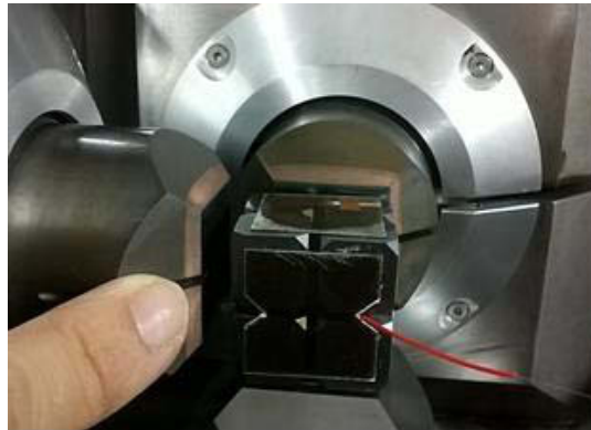
Figure 2.7. Close-up of the 6-8 DIA set-up used for in-situ X-ray diffraction measurements in the Soleil synchrotron. The finger shows the X-ray path. The red wire is the thermocouple.
