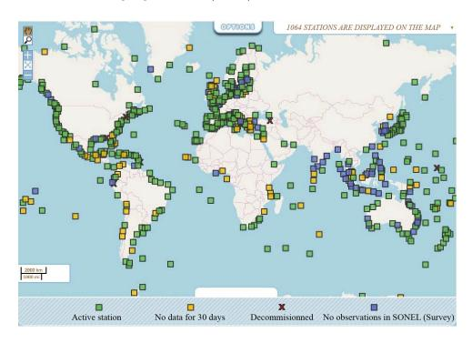
Figure IV.1 – GNSS Observations station for surveying water surface's level of the program GLOSS (Global Sea Level Observing System - http://www.sonel.org/-GPS-.html)
