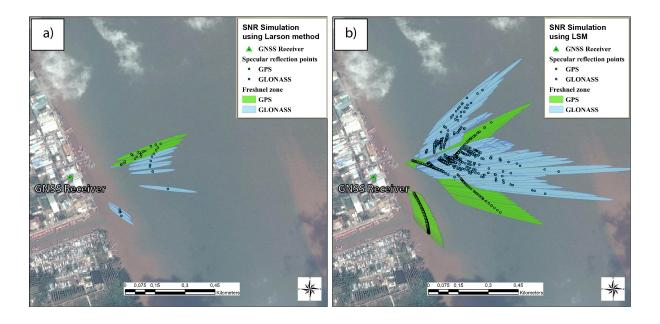
Figure IV.5 – Locations of the specular reflection points and fresnel surface for a GNSS receiver on the top of the Tran De water tower from 23<sup>th</sup> to 30<sup>th</sup> August 2016 (all satellites with elevation angles from 0° to 20°): a) Simulation of SNR multipath using IPT method of Larson et al. (2008b); b) Simulation of SNR multipath using LSM method of Roussel et al. (2015b).
