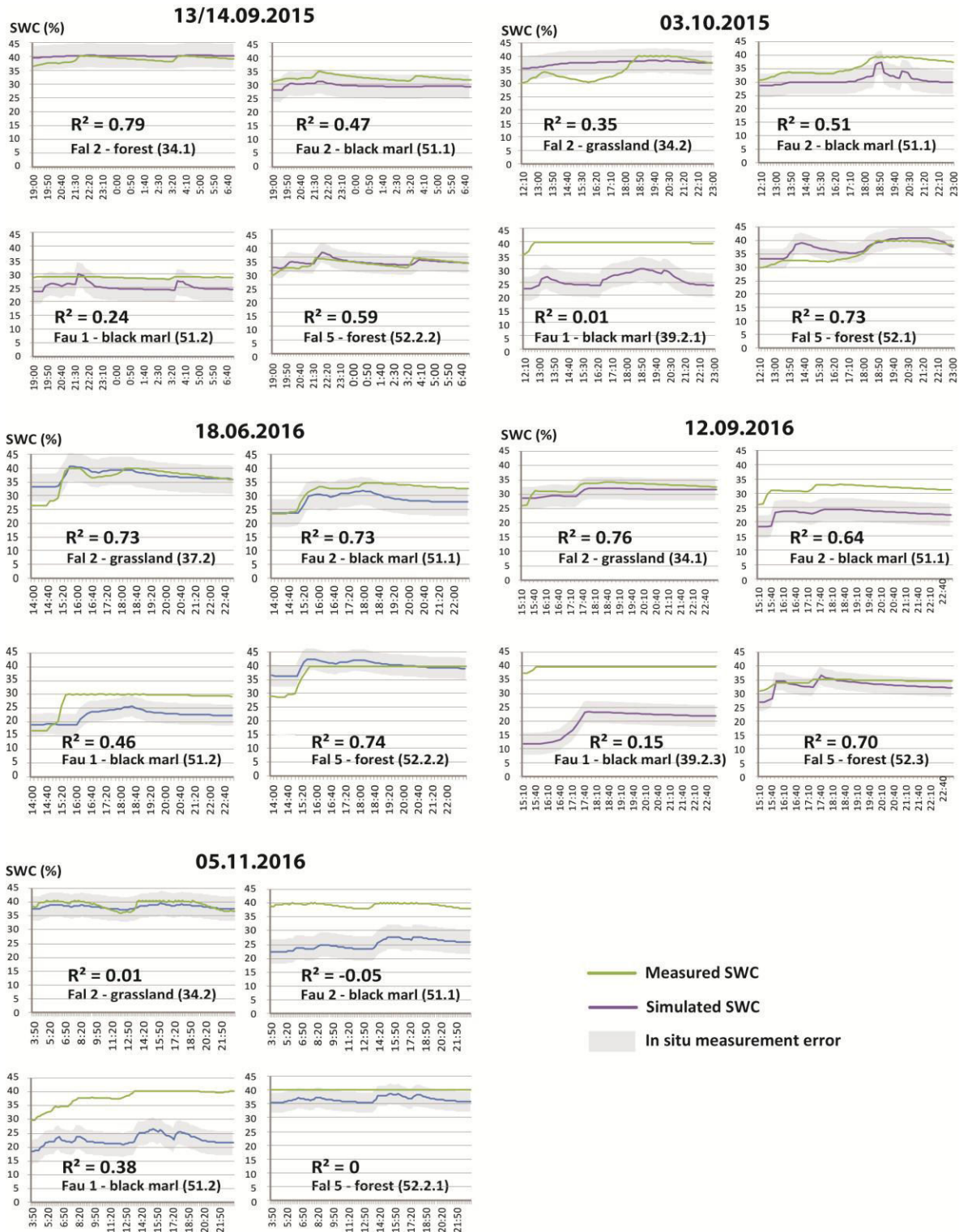
Fig. 4.1.17 : Relationship between measured and estimated SWC. In situ measurement error was estimated at each plot from comparison between SWC values obtained from soil samples and SWC values measured by capacitance probes.
