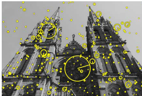
Figure 2.2: Keypoints detected on a photograph of the Cathedral of Clermont Ferrand. SIFT is used to describe the detected keypoints. Yellow circles visualize the position of the keypoint, the scale and orientation of the corresponding descriptor.
