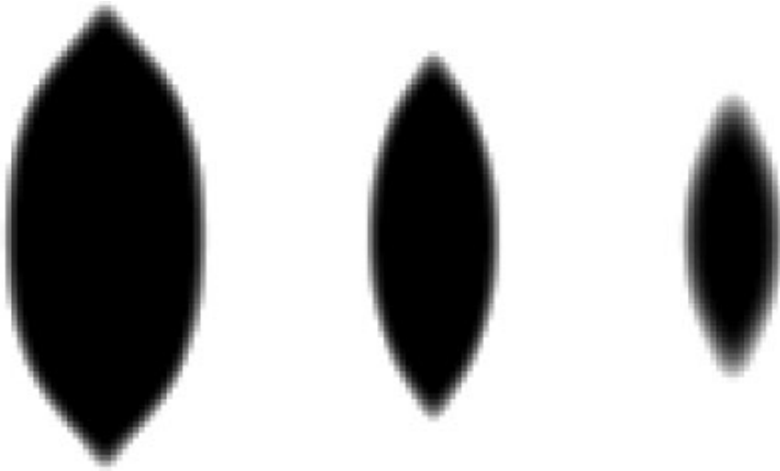
Figure 2.3 – Evolution of a solid obstacle immersed in a cubic domain of Stokes fluid during the topology optimization procedure. A relaxation method is used to minimize the energy dissipated by the fluid. Credits : T. Borrvall and J. Petersson. [30]
