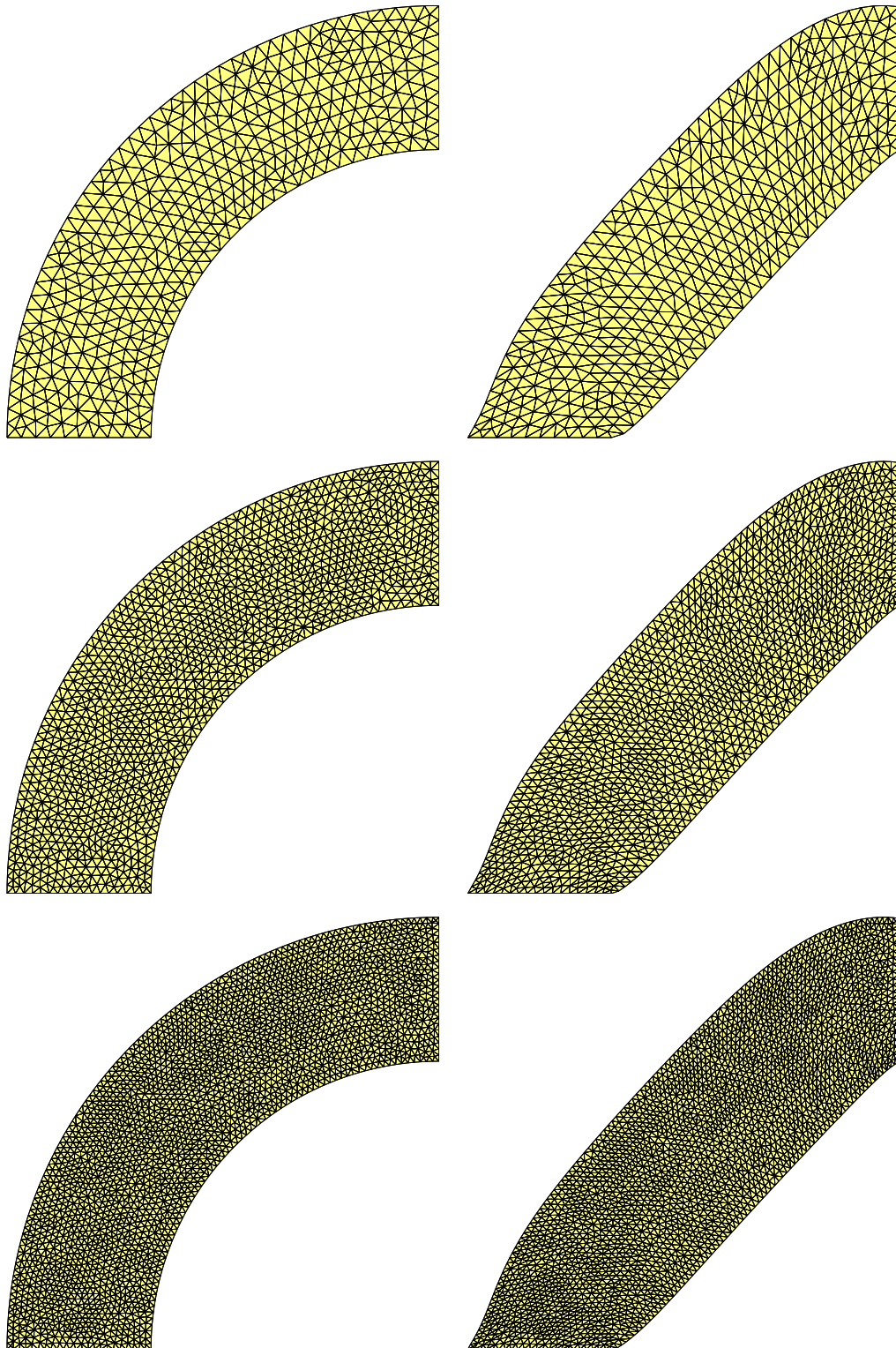
Figure 2.32 – From top to bottom : Initial (left) and final (right) mesh for mesh sizes h = 1/30 , h = 1/50 and h = 1/70 .
