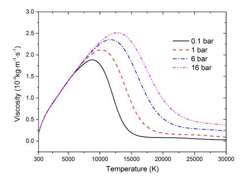
Figure 3-9. Viscosity of CO<sub>2</sub>-N<sub>2</sub> (mixing ratio 7:3) mixtures contaminated by 10% Cu at temperatures of 300 – 30,000 K and at different pressures
