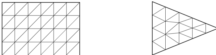
Figure 8: Schematics of meshing a rectangle (left) and an isosceles triangle (right) with the boundary division given.
