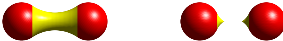
Figure 10: Schematics of a rectangle-shaped toroidal patch (left, yellow) and a double-triangle-shaped toroidal patch (right, yellow) corresponding to two circular SAS circles respectively with radius larger than and smaller than r_p .
