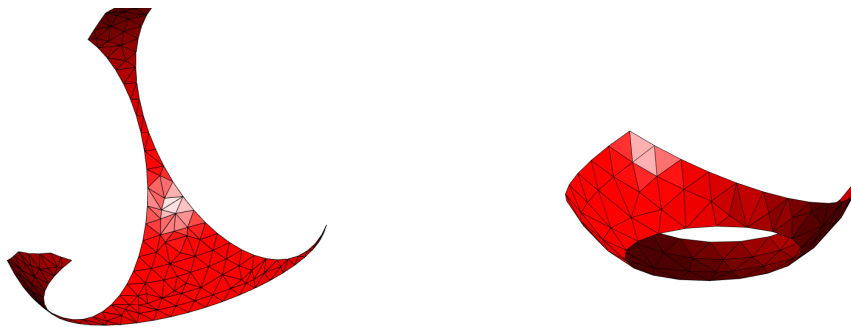
Figure 4: Meshing two spherical patches.
