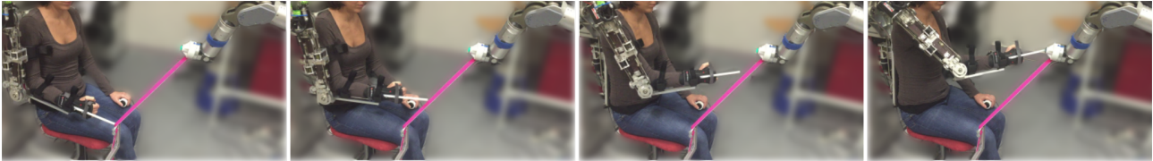
Figure 4.4: Example of path-constrained tracking task (PCT). The four pictures show the motion from the starting position to the WAM button, while performing PCT exercise. The participants were asked to follow the specific endpoint path shown by the rubber band going from the starting position of the ABLE exoskeleton to the WAM end-effector.
